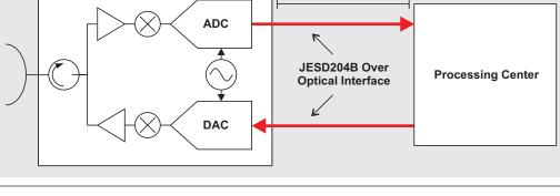
A simplistic board placement shown in Figure 2 demonstrates the feasibility of this architecture in digital L-band, S-band, and potentially C-band radars. The RF paths used
