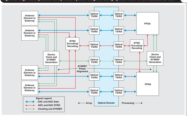
Figure 3. High-level phased-array radar system diagram using optical fiber in the JESD204B link
