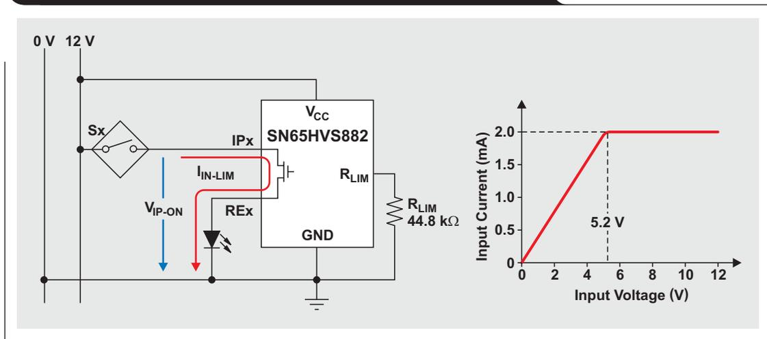
**Figure 4. Switch ON condition:  $V_{IN-ON} = 12\text{ V}$ ,  $I_{IN-LIM} = 2\text{ mA}$**
