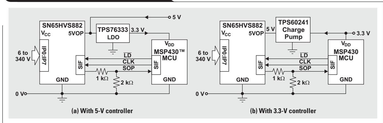
input while leaving the normal  $V_{CC}$  supply pin floating. Figure 9 shows two back-supply options for interfacing to a 3.3-V controller. In Figure 9a, the 5-V system supply powers the DIS directly but requires an LDO to supply the controller. In Figure 9b, a 3.3-V supply powers the controller directly but requires a charge pump to boost the supply voltage to the required 5-V level of the DIS.
