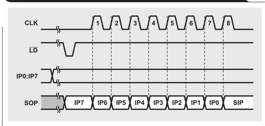
Designing input modules with a high channel count is possible by daisy-chaining multiple DIS devices. In this case the serial output of a leading device is connected with the serial input of a following device. Figure 7 shows the simplicity of a daisy-chained, 64-channel digital-input module requiring only three interface lines.
