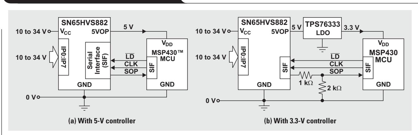
**Figure 9. Back-supplied digital-input system**
