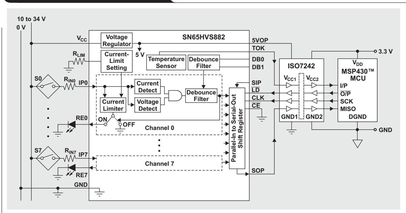
fixed reference voltage. If both comparator outputs are logic high, a programmable debounce filter checks whether the new input status is caused by a short but strong noise transient, or whether the signal presence outlasts the debounce time and thus presents a true input signal.
