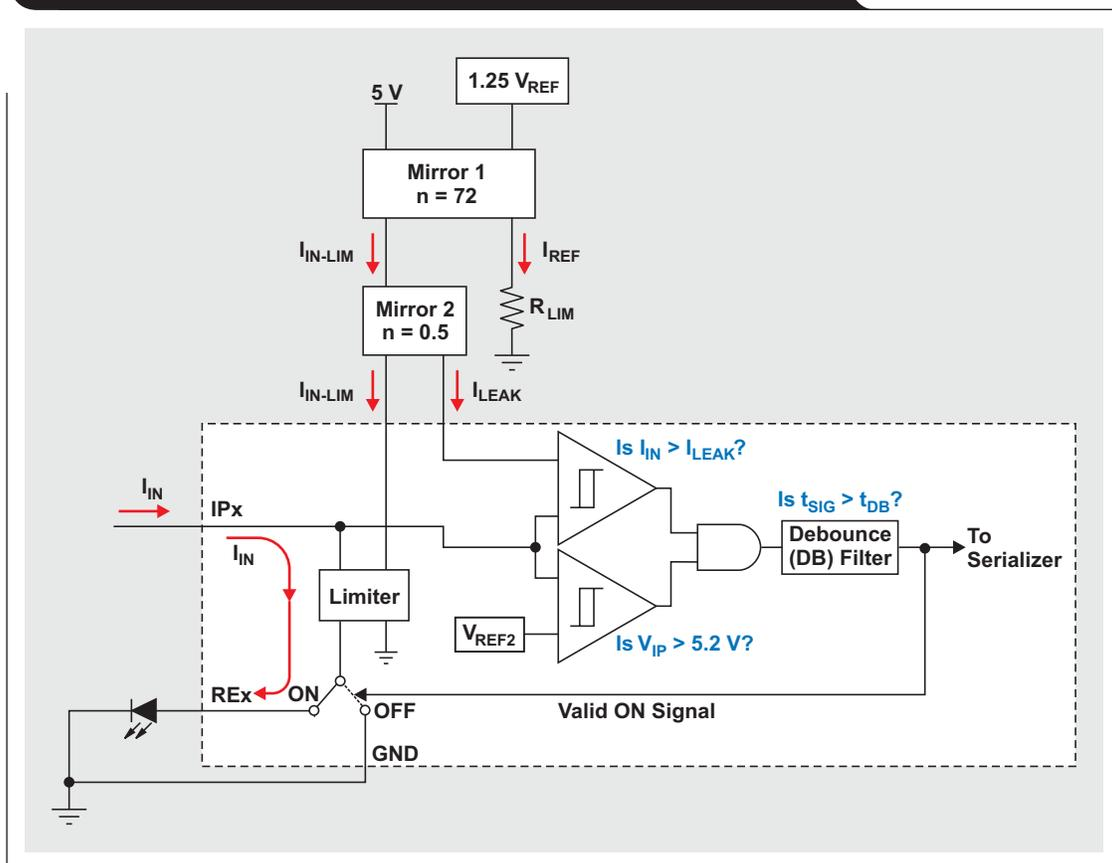
input causes no damage to the device. With  $V_{IP-ON} = 5.2\text{ V}$ , the ON threshold lies almost in the middle of the 12-V input-voltage range. Figure 3 shows the schematic of this simple circuit design. With the low-current LED indicator requiring a forward current of  $I_{IN-LIM} = 2\text{ mA}$ ,  $R_{LIM}$  is determined via Equation 2 to be  $45\text{ k}\Omega$ , with the closest 1% value being  $44.8\text{ k}\Omega$ .
