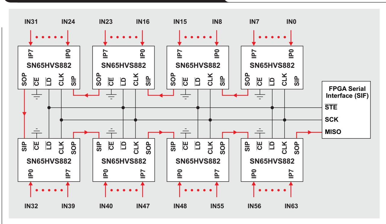
**Figure 8. Bus-powered digital-input system**
