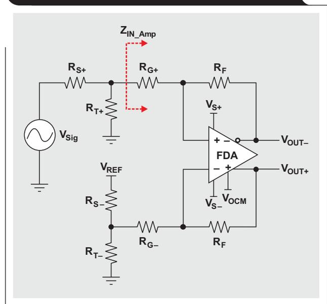
If we choose to keep  $R_F$  the same on both sides of the FDA, then we need to balance the gain-setting resistances by setting
