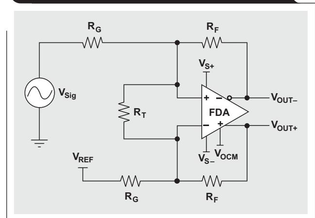
is accomplished by keeping the parallel combination equal to  $R_G$  while simultaneously setting the voltage divider to provide the input common-mode voltage at no load.
