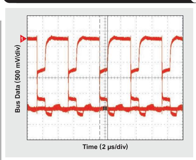
**Figure 7. Addition of 0.5 m to bus length**
