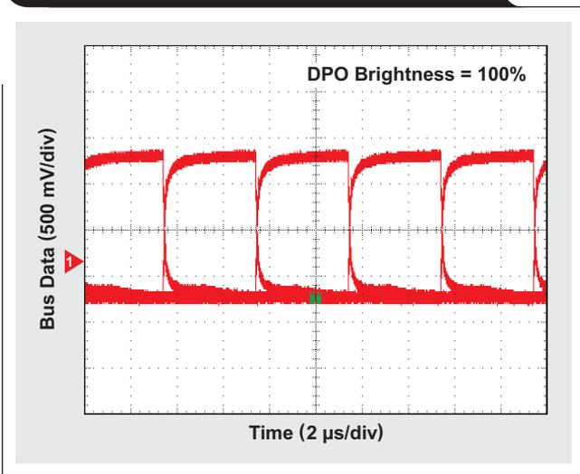
**Figure 6. Reflected-wave distortion by multiple dominant bits**
