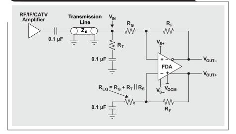
Figure 6 shows the case where the source is ground-referenced and  $R_S$  and  $R_T$  are combined with  $R_G$  into one resistor of equivalent value,  $R_{EQ} = R_G + R_T \parallel R_S$ , which is tied to ground. We will base the analysis of the input impedance on this circuit.
