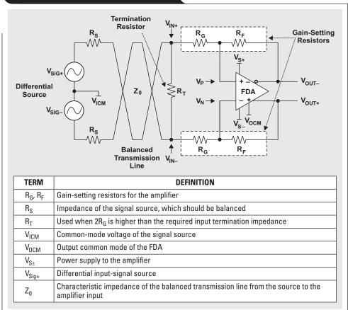
nated with that impedance. No matter what impedancematching scheme is chosen, the termination impedance to implement must be accurately calculated.
