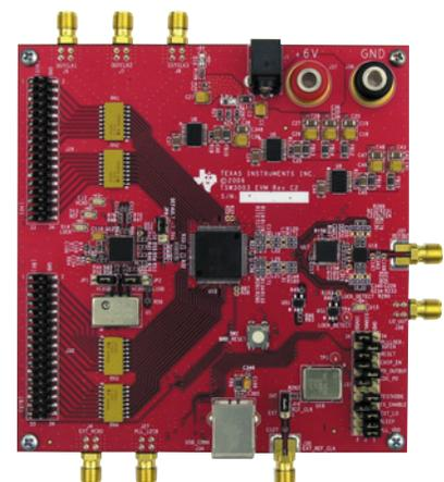
The CDCM7005 is a high-performance, low-jitter clock solution that synchronizes an onboard voltage-controlled crystal oscillator (VCXO) to a reference clock. Once the proper reference frequency and programming are applied, the CDCM7005 supplies two clock sources to the DAC and an additional three outputs for external equipment.
