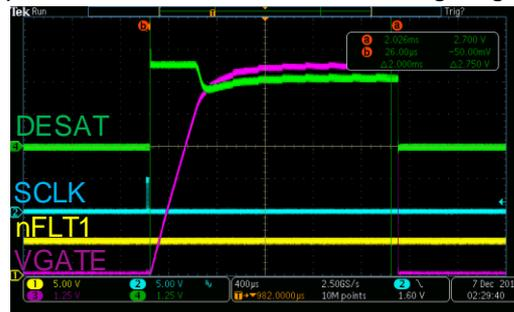
*$V_{GTH}$  is accurate measure of health of external power switch
