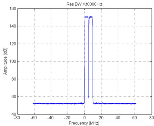
Figure 11. FFT of Two Carrier WCDMA TM1 Pattern
