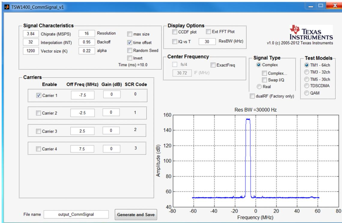
Figure 8. TSW1400 CommSignal User Interface
