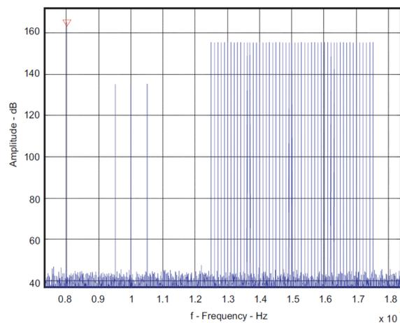
Figure 6. Magnified Spectral Plot of Three Tone Group
