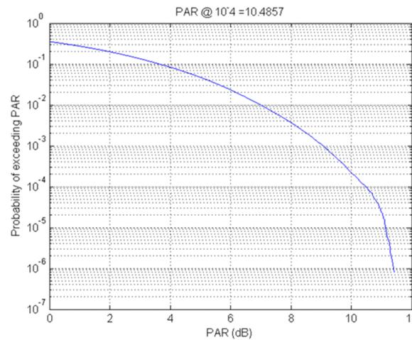
Figure 12. CCDF of Two Carrier WCDMA TM1 Pattern
