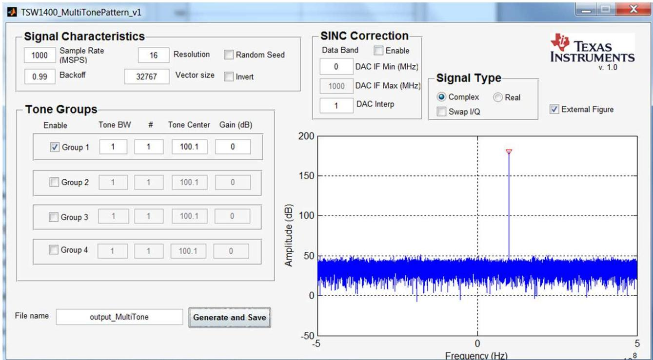
Figure 4. TSW1400 MultiTonePattern User Interface
