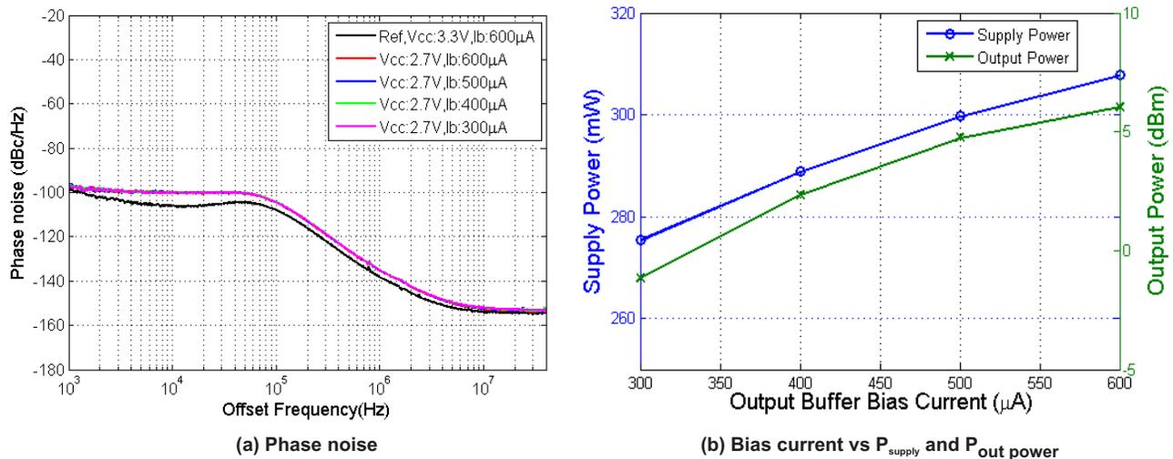
**Figure 3. (a) Phase Noise Response at  $V_{CC}$  2.7 V for 900 MHz and Different Output Buffer Bias Current Supply. (b) Supply Power and RF Output Power vs Output Buffer Bias Current at 900 MHz and  $V_{CC}$  2.7 V**
