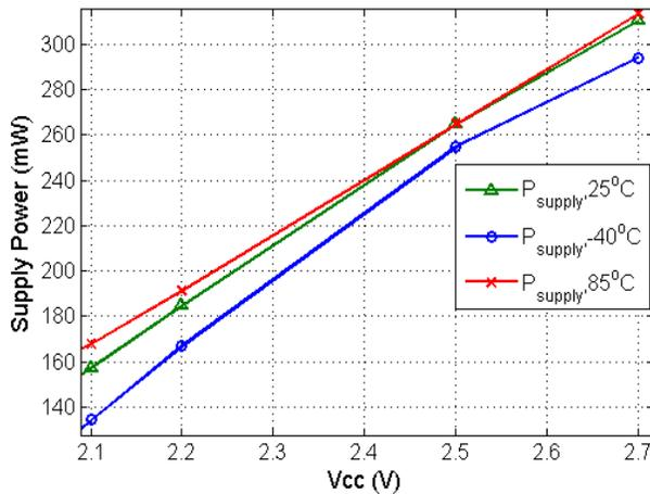
(c)  $V_{CC}$  vs supply power
