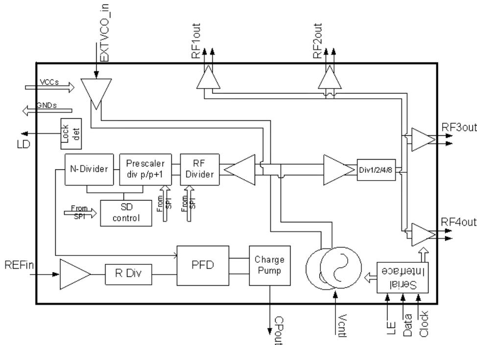
**Figure 1. TRF3765 Block Diagram**
