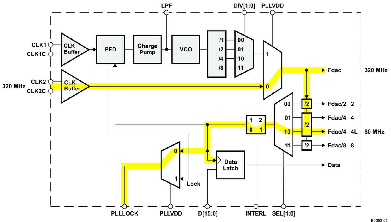
Figure 3. Example 1: External Clock, Non-Interleaved Data
