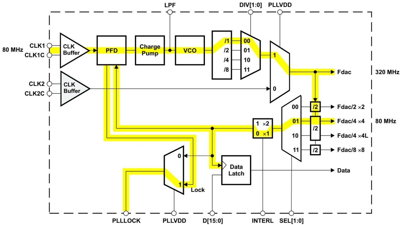
Figure 5. Example 3: PLL Mode Non-Interleaved Data
