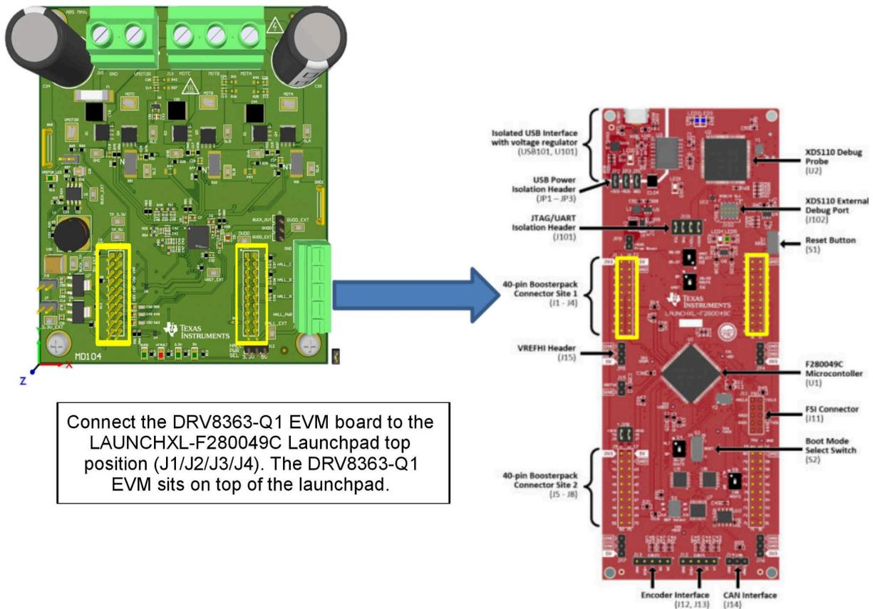
Figure 2-2. DRV8363-Q1EVM Mating to LAUNCHXL-F280049C
