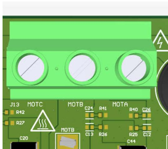
**Figure 2-5. Motor Phase Connector (J13)**
