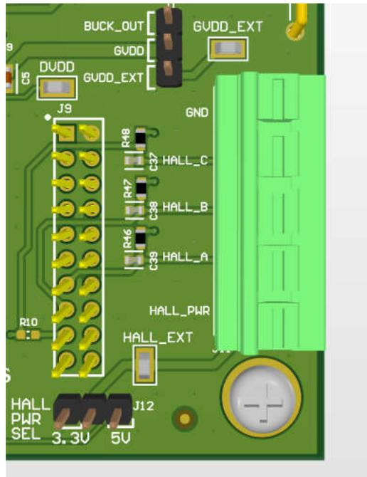
**Figure 2-4. Hall Sensor Input and Power Connections (J11)**
