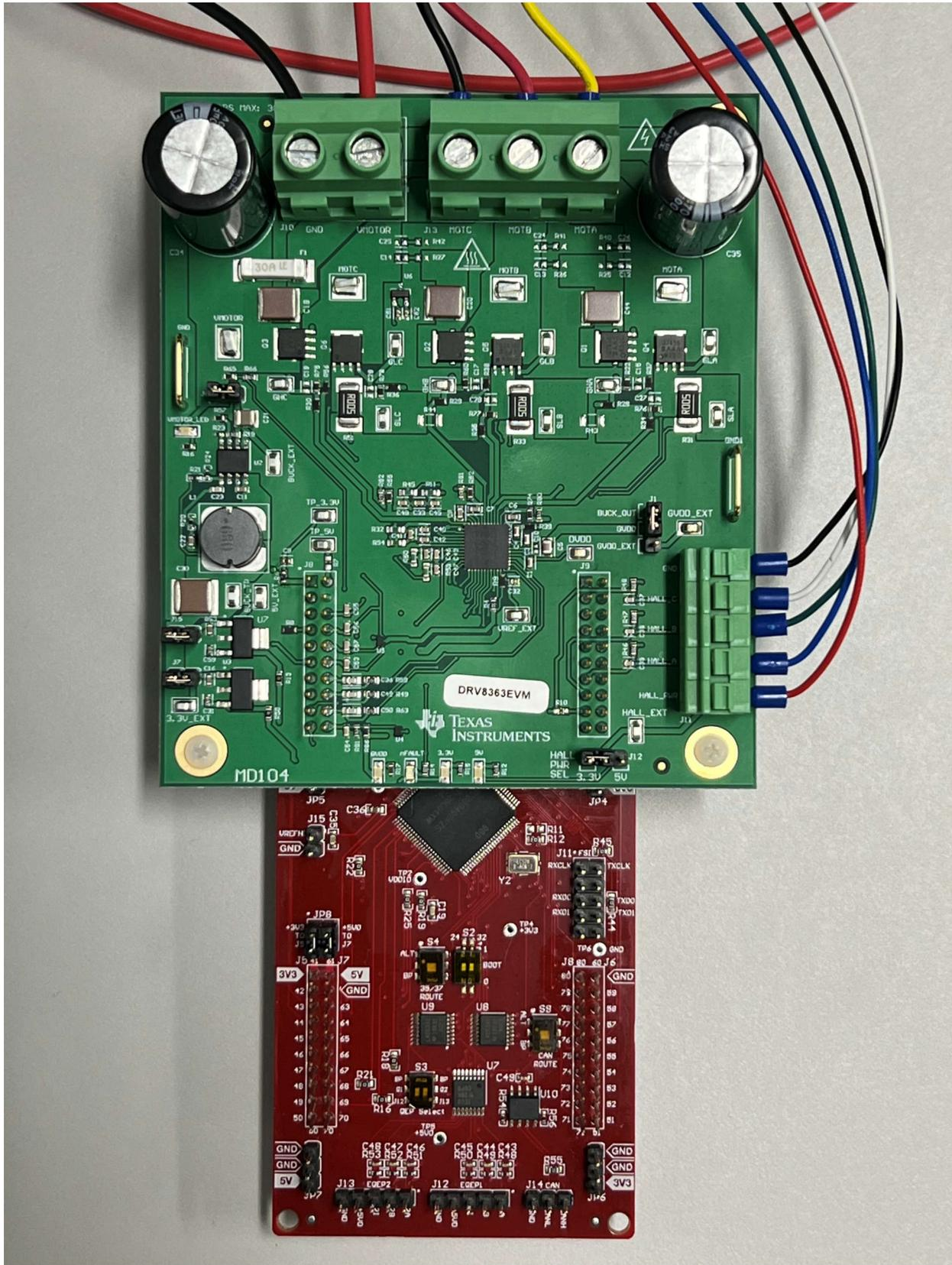
Figure 2-8. DRV8363-Q1EVM connected with Launch Pad
