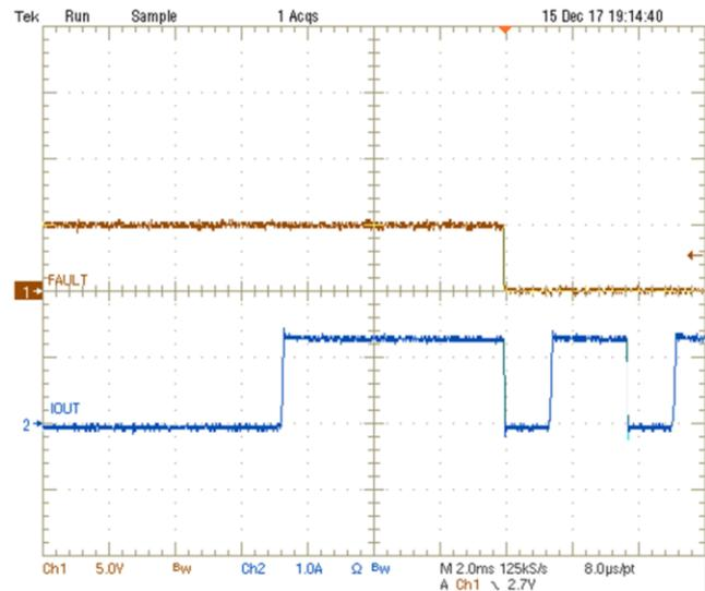
Figure 4. TPS25221DBVEVM Short-Circuit Output Current and FAULT Status With J3 Shorting Jumper Absent
