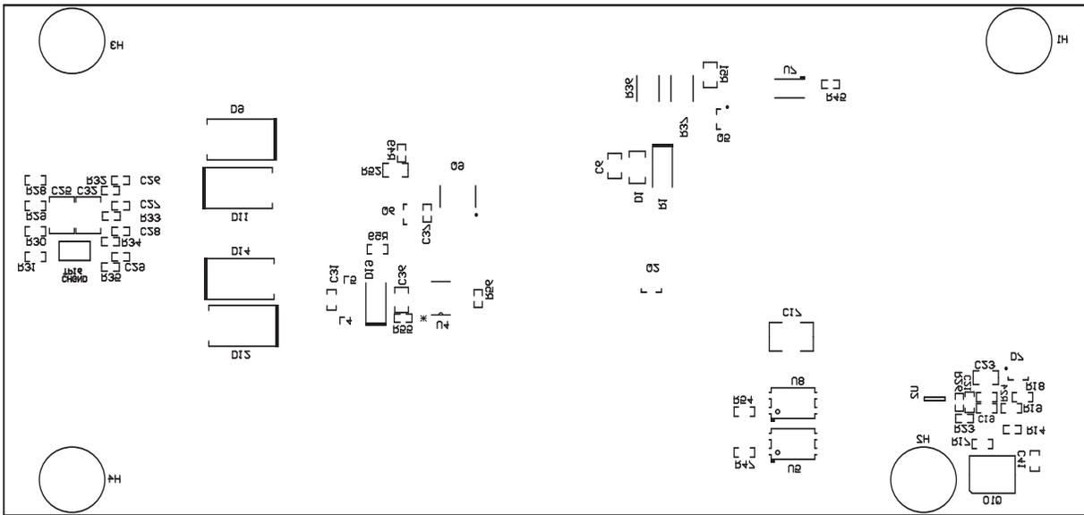
**Figure 13. Bottom Component Placement**
