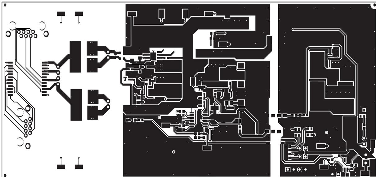
Figure 9. Top Side Routing
