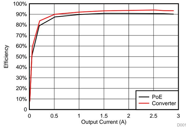
Figure 7. Efficiency of the TPS2378EVM-602
