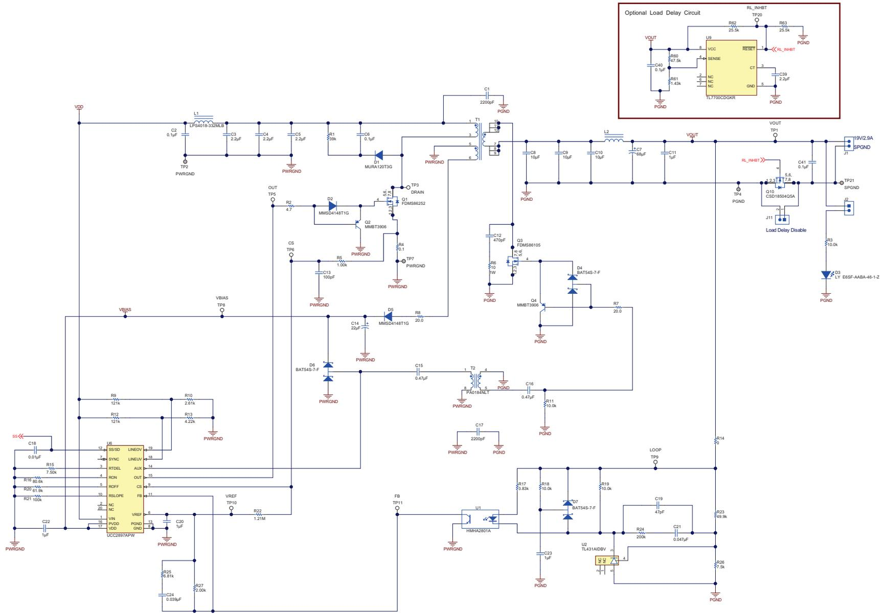
Figure 3. TPS2378EVM-602 DCDC Converter Section
