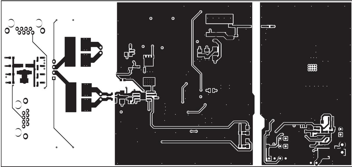
**Figure 12. Bottom Side Routing**
