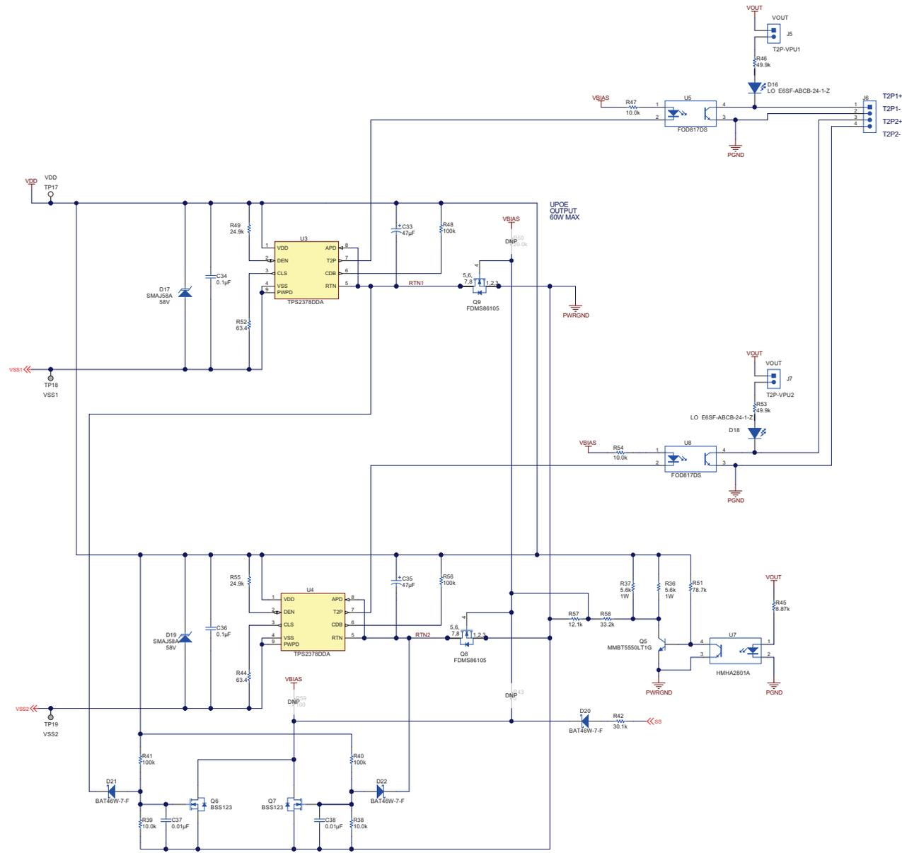
Figure 2. TPS2378EVM-602 Dual PD section
