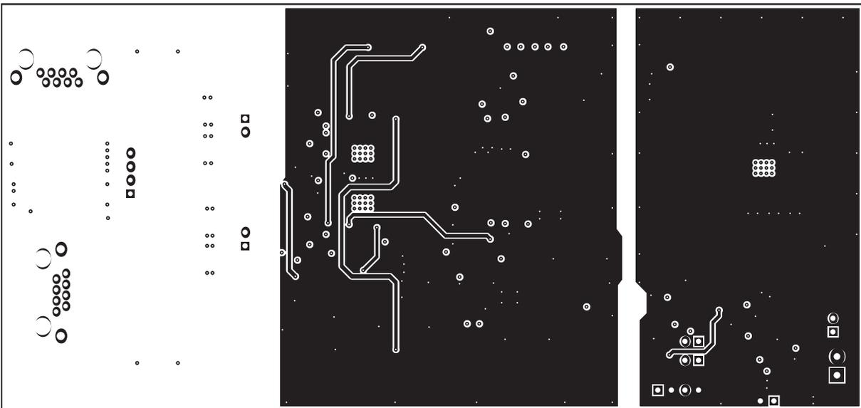
Figure 11. Layer 3 Routing
