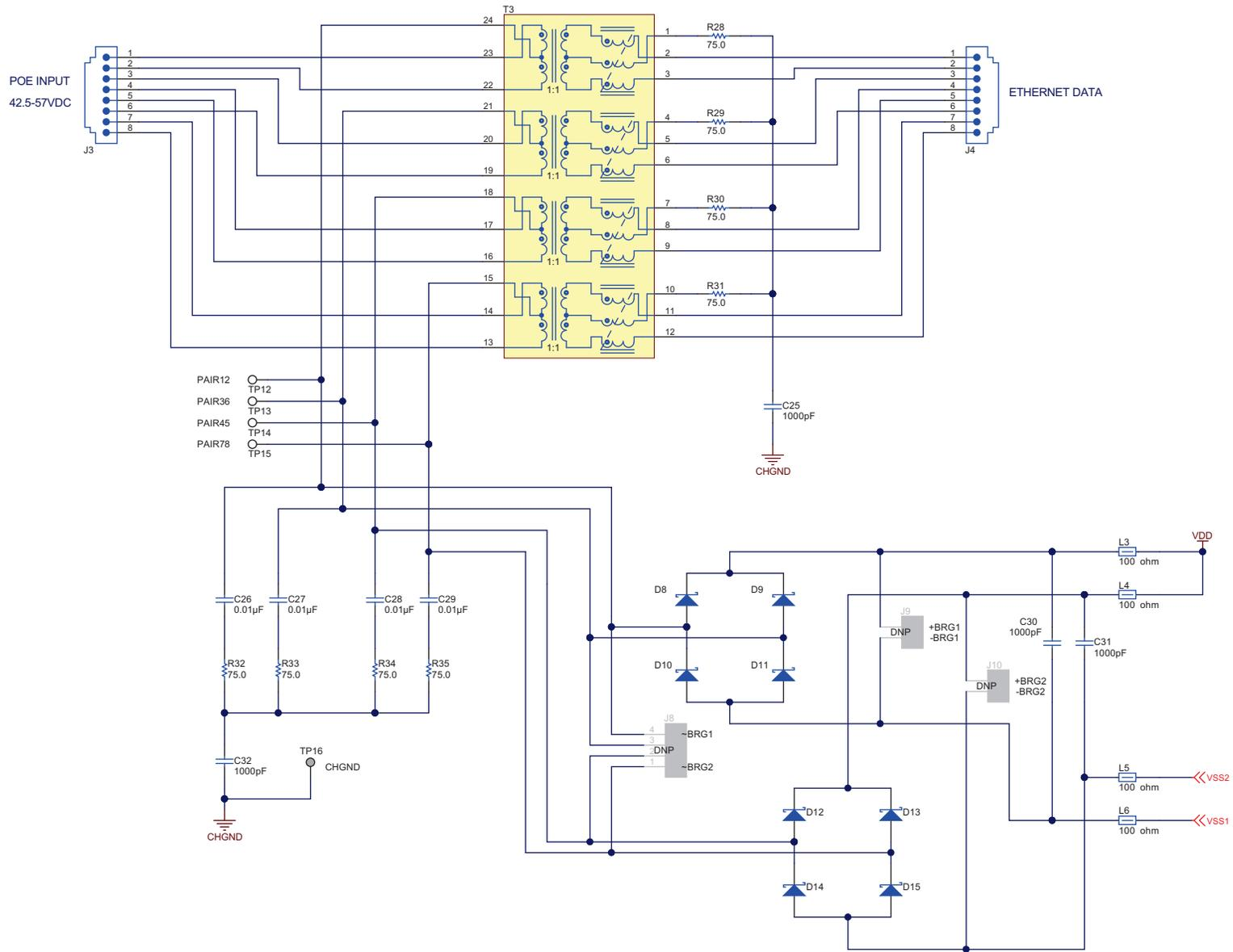
Figure 1. TPS2378EVM-602 PD Front-End Schematic
