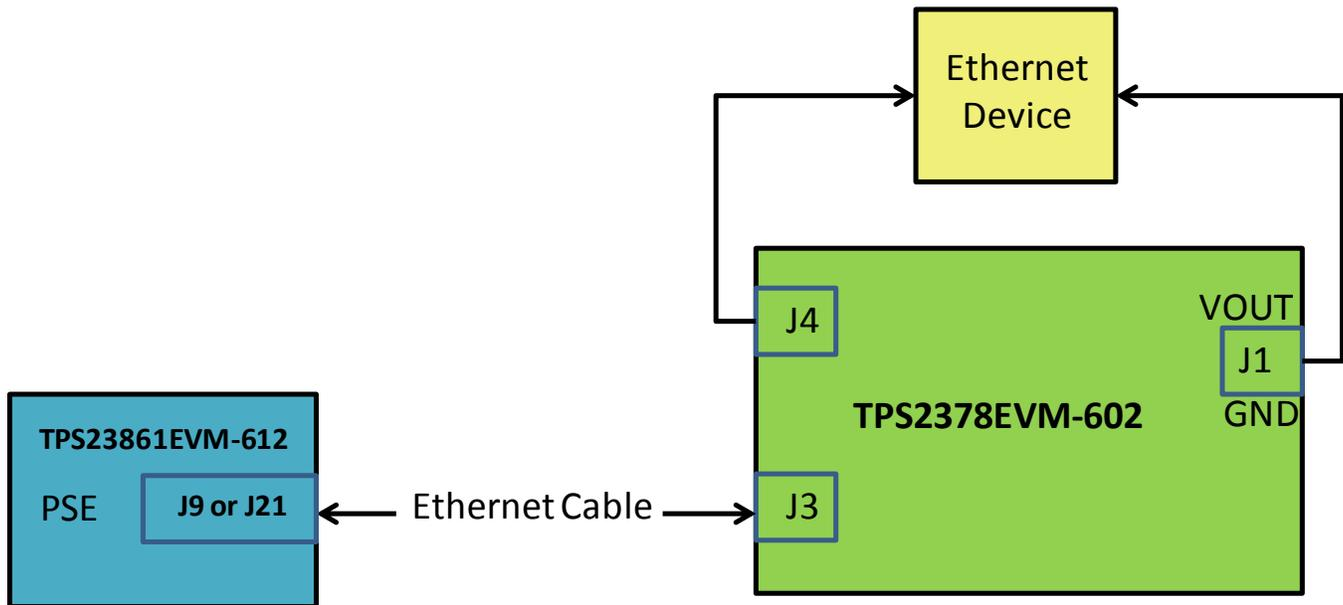
Figure 4. Typical TPS2378EVM-602 Test Setup
