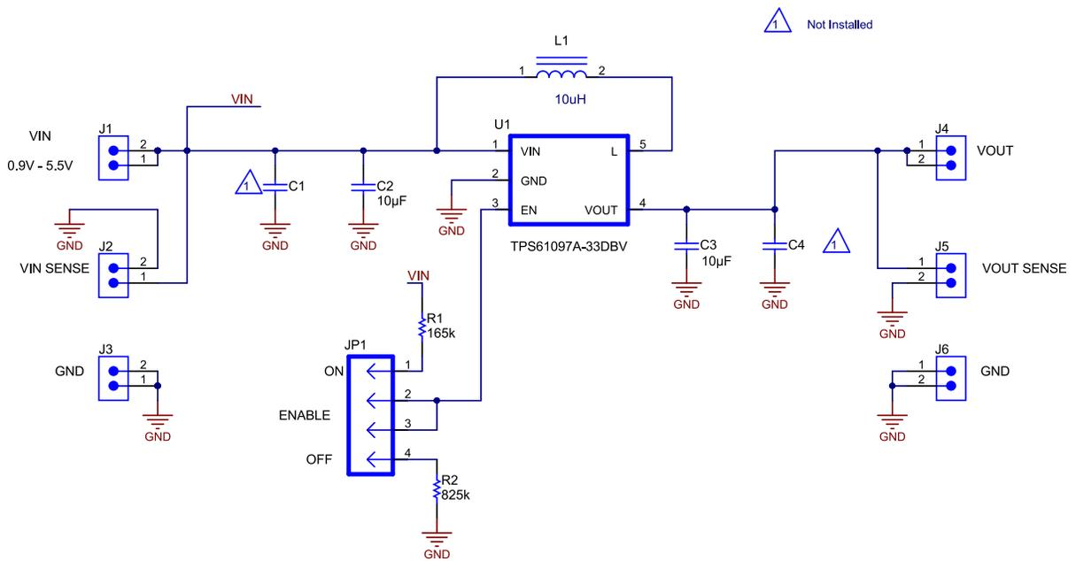
Figure 4. TPS61097AEVM-073 Schematic
