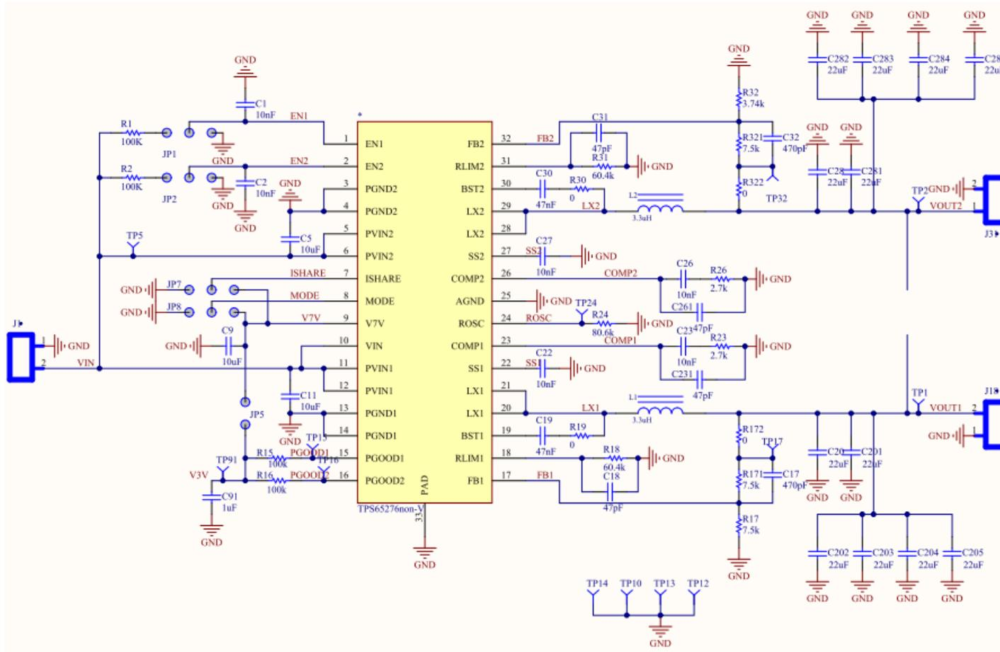
Figure 1. TPS65279 Schematic
