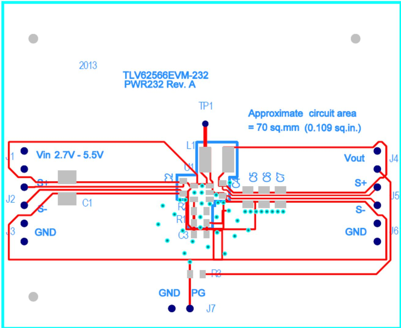
Figure 2. Assembly Layer
