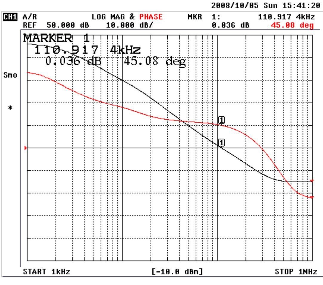
Figure 1. Bode Plot with  $V_{IN} = 3.6\text{ V}$ ,  $V_{OUT} = 1.8\text{ V}$ ,  $I_{OUT} = 1\text{ A}$
