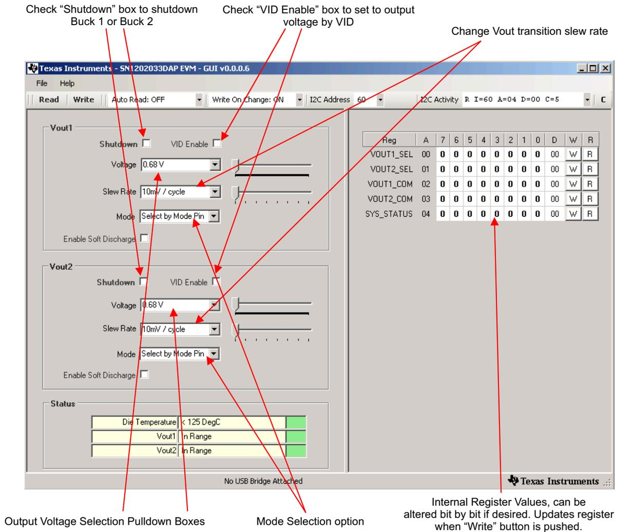
**Figure 5-3. Screen Capture of TPS65279V Software GUI Interface**
