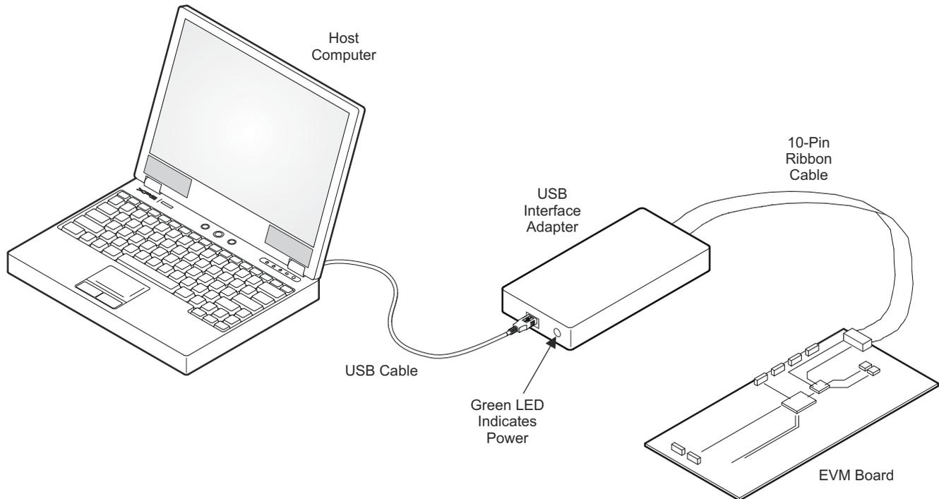
**Figure 5-2. USB Interface Adapter Quick Connection Diagram**
