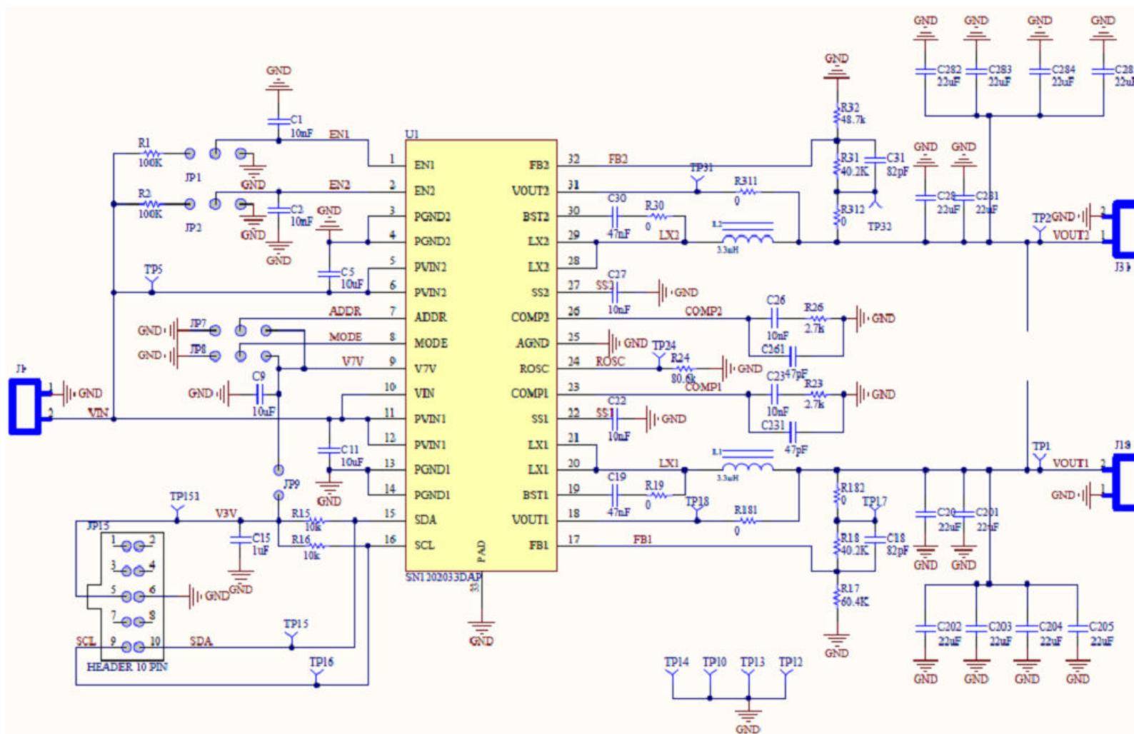
Figure 3-1. TPS65279V Schematic
