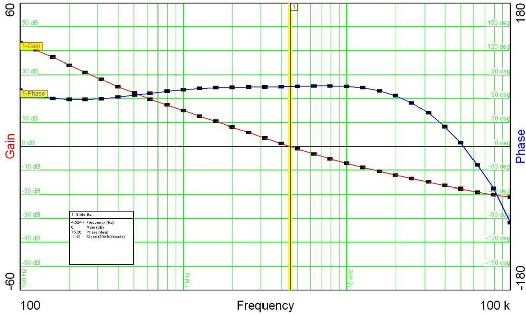
The figure below is the loop gain of the converter with a 48V input and 180mA load. The bandwidth is 1.6 KHz, the phase margin is 69 degrees, and the gain margin is 34 dB.
