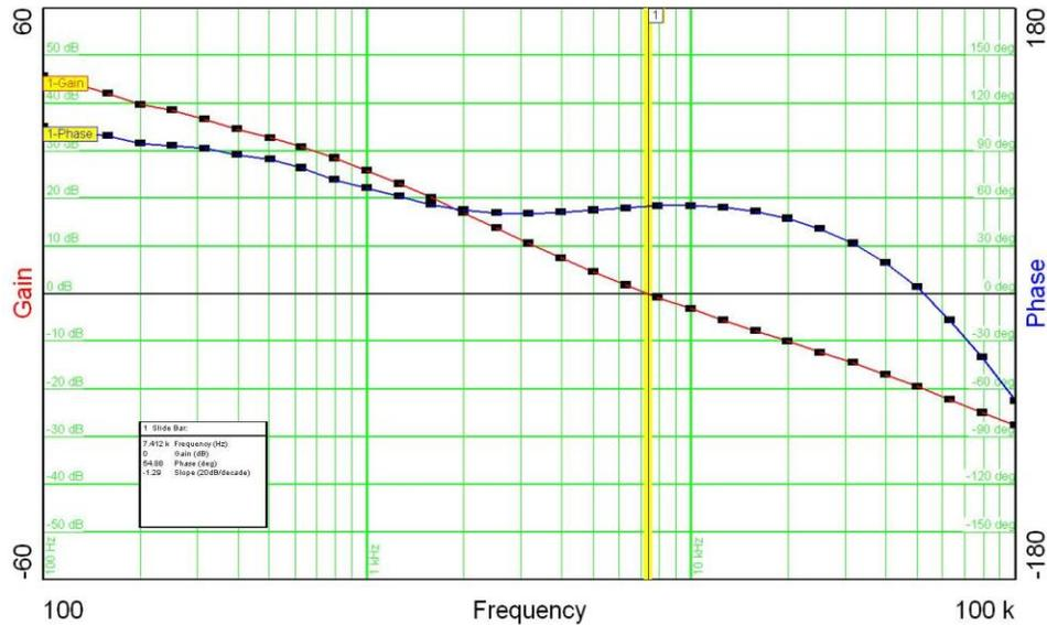
The figure below is the loop gain of the converter with a 48V input and 90mA load. The bandwidth is 3.5 KHz, the phase margin is 43 degrees, and the gain margin is 33 dB.
