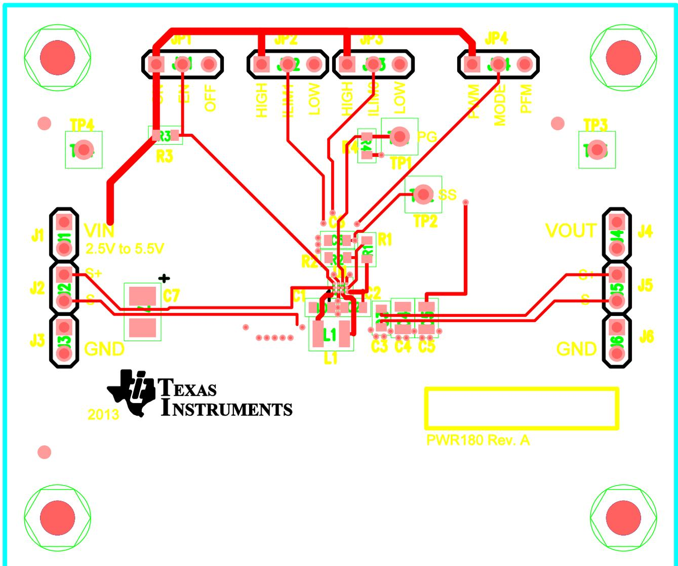
Figure 2. Assembly Layer
