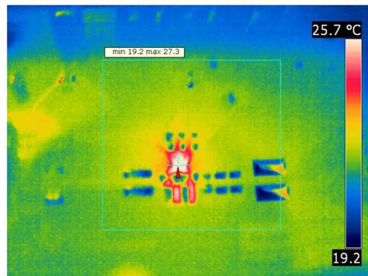
**Figure 1. Thermal Performance (Vin = 5.5 V, Load = 500 mA)**
