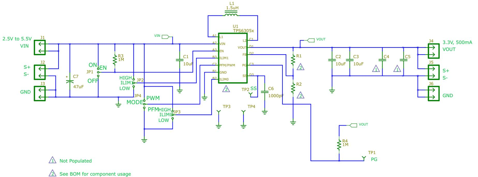
Figure 5. TPS6305xEVM-180 Schematic
