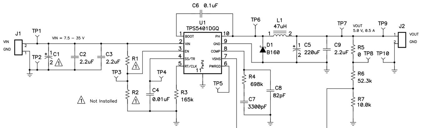
Figure 14. TPS5401EVM-708 Schematic
