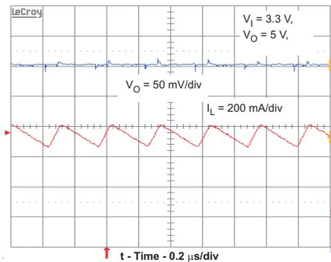
Figure 8. TPS61252 EVM Output Voltage Ripple at Overload
