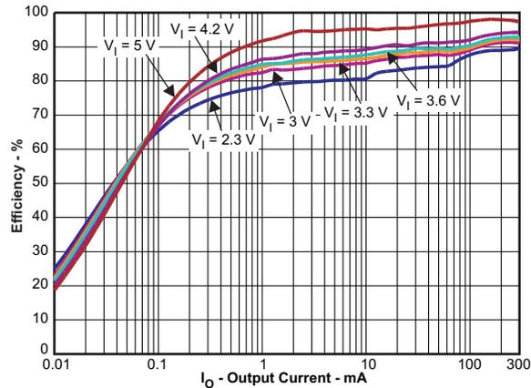
Figure 2. TPS61252 EVM Efficiency vs Load Current
