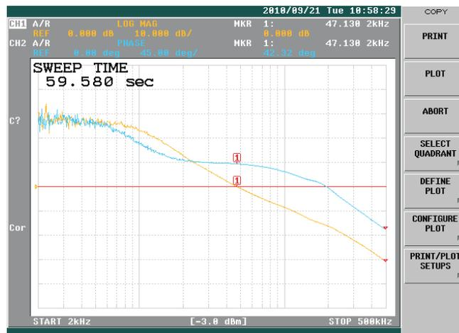
Figure 9. TPS61252 EVM Gain and Phase vs. Frequency
