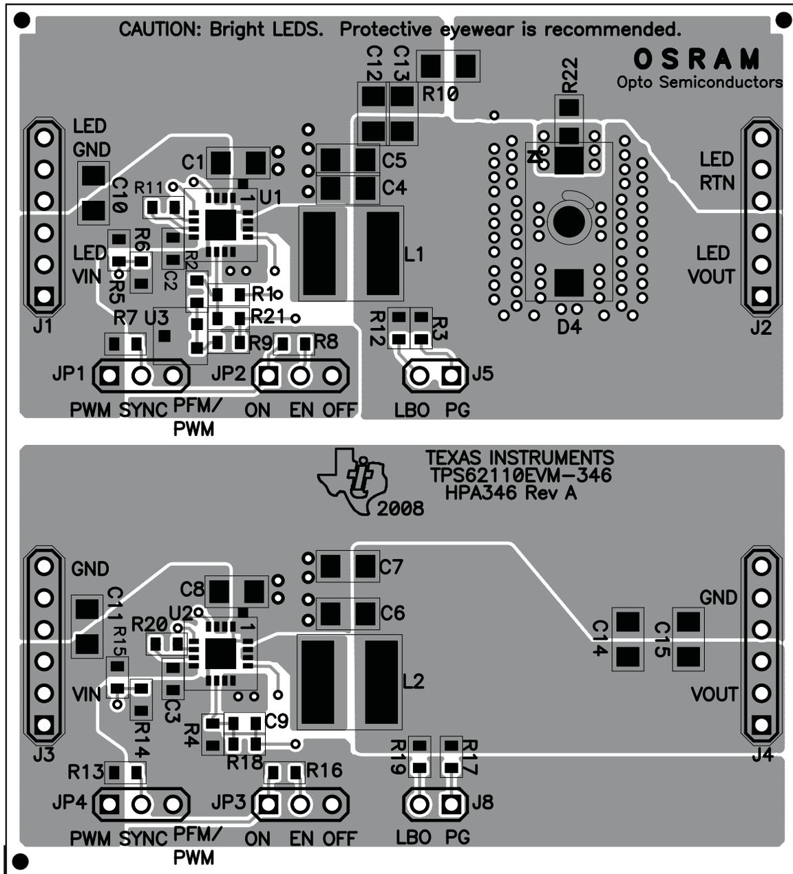
Figure 4. Assembly Layer
