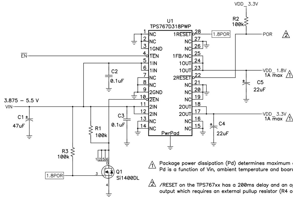
⚠ Package power dissipation (Pd) determines maximum current. Pd is a function of Vin, ambient temperature and board layout.
