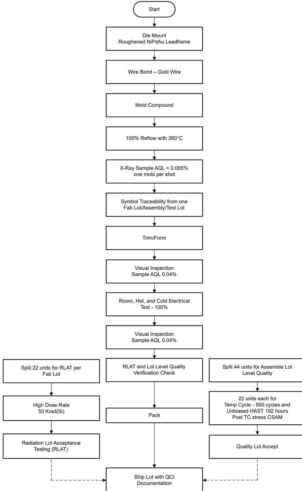
**Figure 2-1. TPS7H3302-SEP Space Enhanced Plastic Production Flow Chart**
