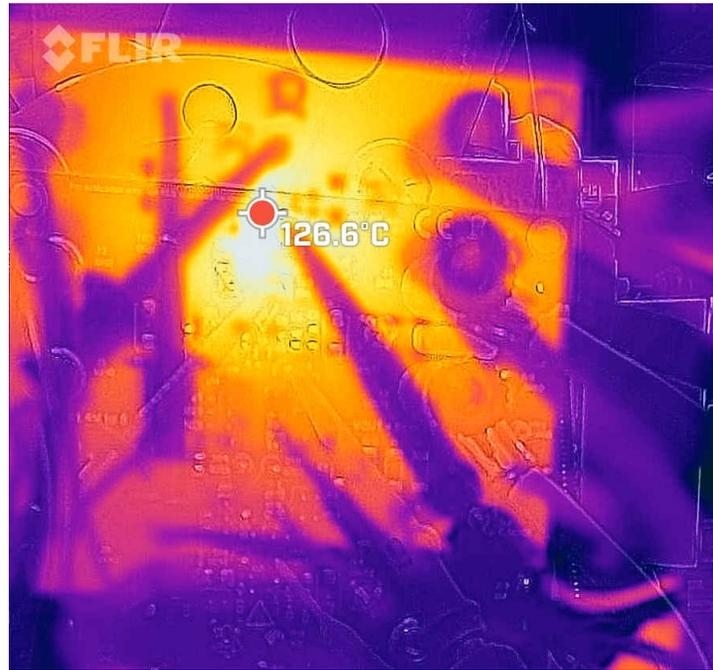
Figure 3-3. TPS7H2221-SEP Thermal Image for SEL
