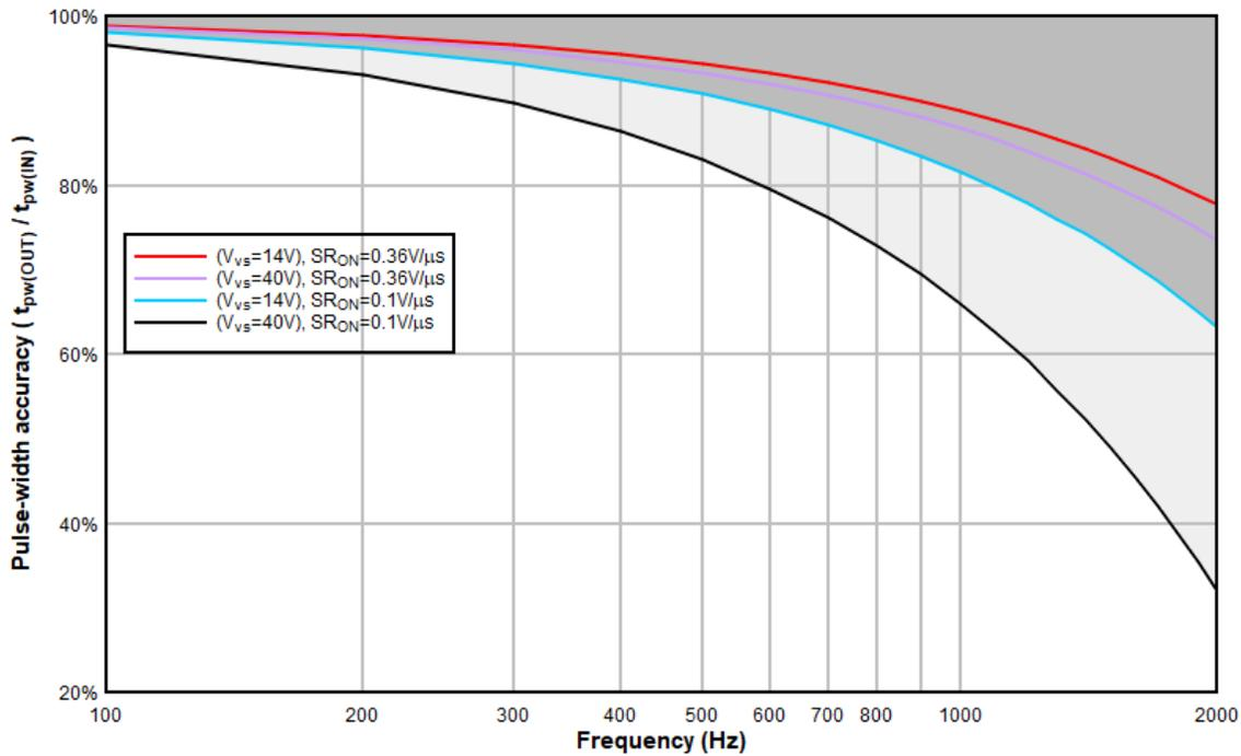
Figure 3-7. Input-to-Output PW Accuracy Over Supply Voltage, Considering Slew Rate and Delay Mismatch
