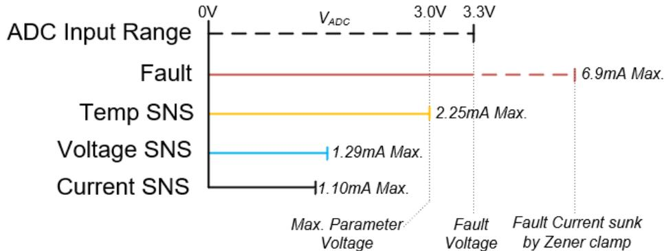
**Figure 4-2. ADC Range Allocation**
