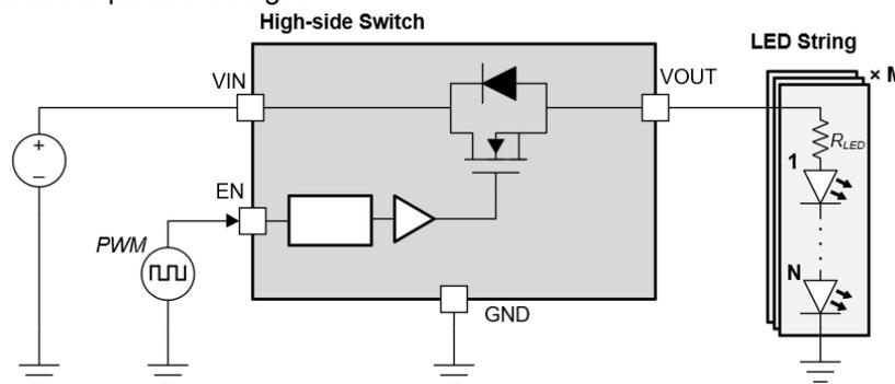
**Figure 3-9. High-Side Switch Driving LED Load**
