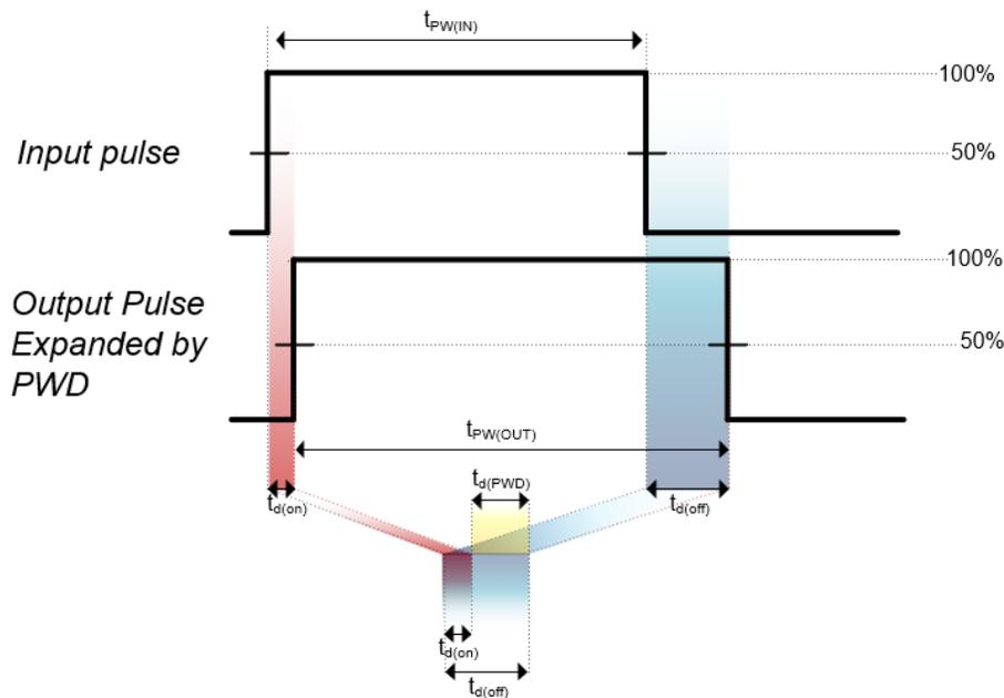
**Figure 3-2. Pulse-Width Distortion Timing Definition**
