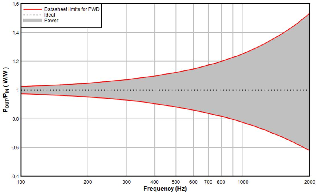
**Figure 3-6. Potential Load Power Variation for TPS4H000, Normalized**
