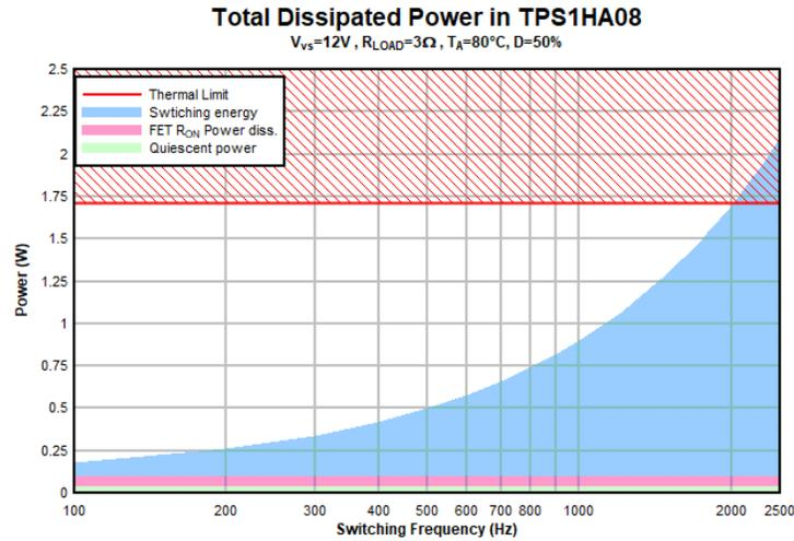
**Figure 2-1. Power Dissipation Sources in TPS1HA08**
