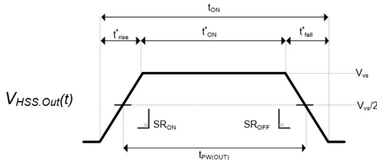
Figure 3-8. Timing Definition for Resistor Power Analysis
