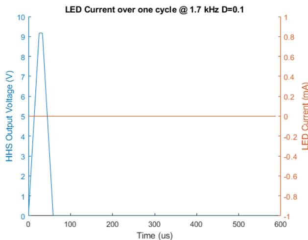
**Figure 3-14. TPS1HA08-Q1 Driving LED, Insufficient Pulse-Width,  $f = 1.7 \text{ kHz}$  ,  $D = 10\%$**
