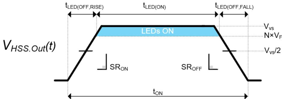
**Figure 3-11. Timing Definitions for LED Power Analysis**
