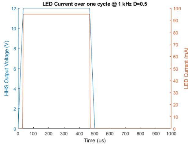
**Figure 3-12. TPS1HA08-Q1 Driving LED String Sample Design,  $f = 1 \text{ kHz}$  ,  $D = 50\%$**
