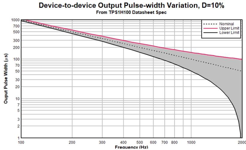
**Figure 3-5. Device-to-Device Output Pulse-Width Variation, D = 10%**
