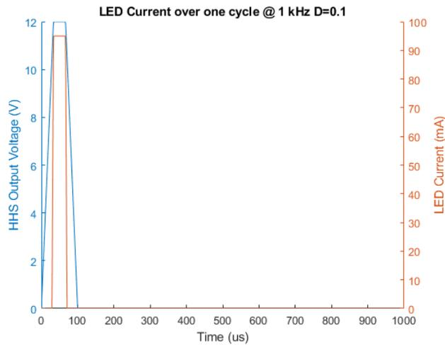
**Figure 3-13. TPS1HA08-Q1 Driving LED String Sample Design,  $f = 1 \text{ kHz}$  ,  $D = 10\%$**
