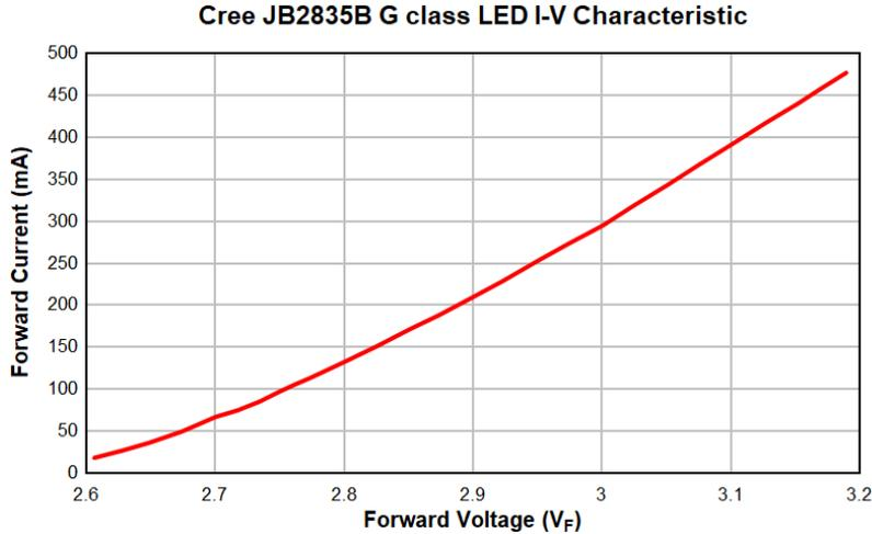
**Figure 3-10. Cree JB82835 0.5-W LED I-V Characteristic**
