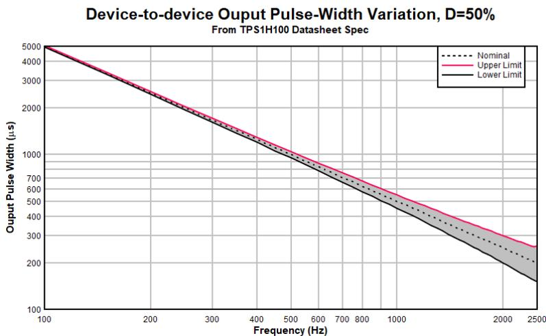
Figure 3-4. Device-to-Device Output Pulse-Width Variation, D = 50%
