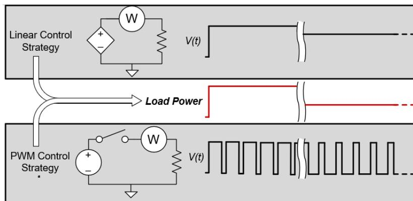
**Figure 1-1. PWM and Linear Control of Load Power**
