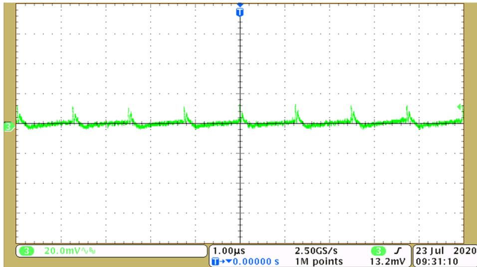
Figure 3-3. Output Voltage Ripple at 1mA load Current ( $V_{in}=3.3\text{ V}$ ,  $V_{out}=-90\text{ V}$ )
