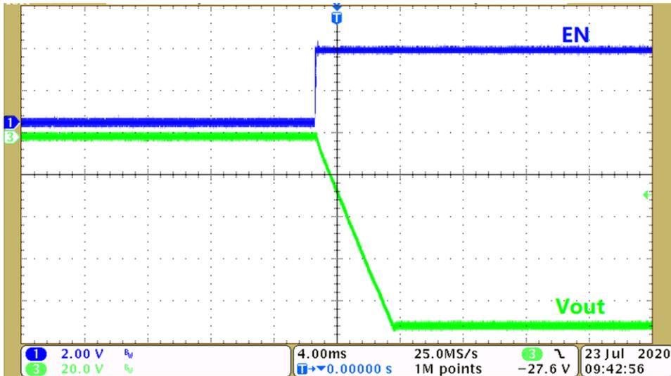
**Figure 3-2. Enable Start-up Waveform (Vin=3.3 V, Vout=-90 V)**
