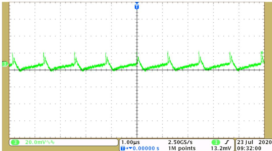
Figure 3-4. Output Voltage Ripple at 2mA load Current ( $V_{in}=3.3\text{ V}$ ,  $V_{out}=-90\text{ V}$ )
