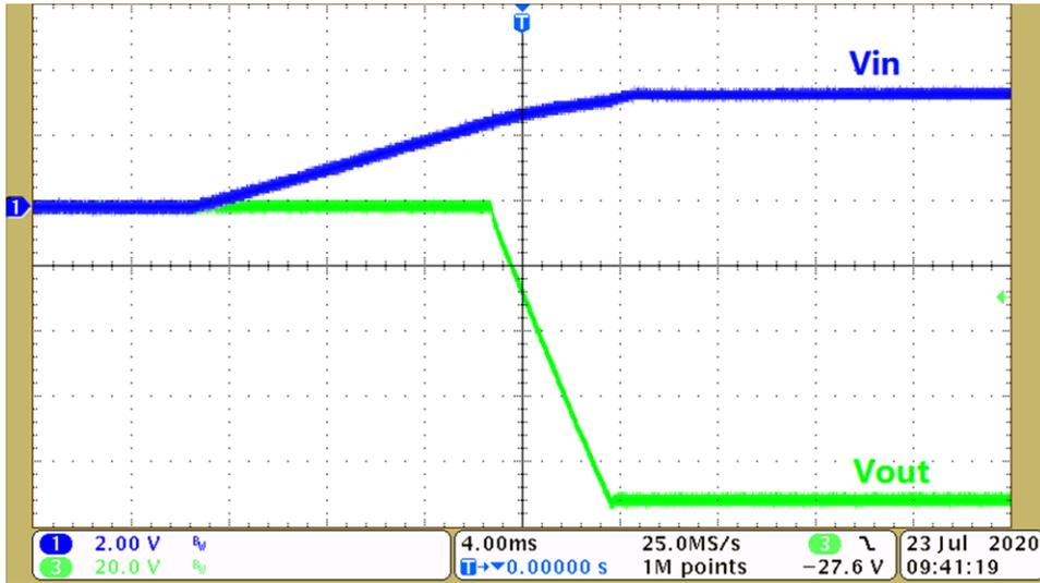
**Figure 3-1. Input Voltage Start-up Waveform (Vin=3.3 V, Vout=-90 V)**
