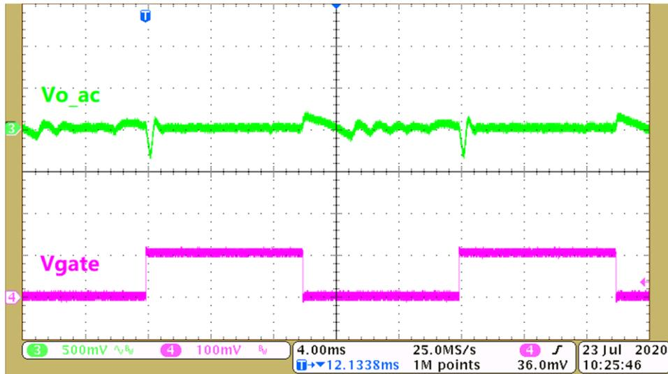
Figure 3-5. Load Dynamic Performance at 2mA Load Step ( $V_{in}=3.3\text{ V}$ ,  $V_{out}=-90\text{ V}$ )
