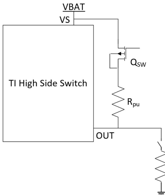
Figure 3-1. External Circuitry Used to Minimize Leakage Current and Identify Open Load
