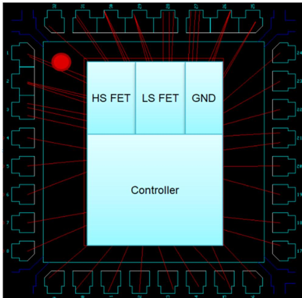
**Figure 1. Inner Function Module and Pinout of the TPS2583X**
