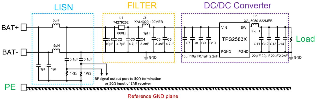
Figure 3. Recommended Parameters for Input Filter, Input Capacitor, Freewheeling Inductor, and Output Capacitor
