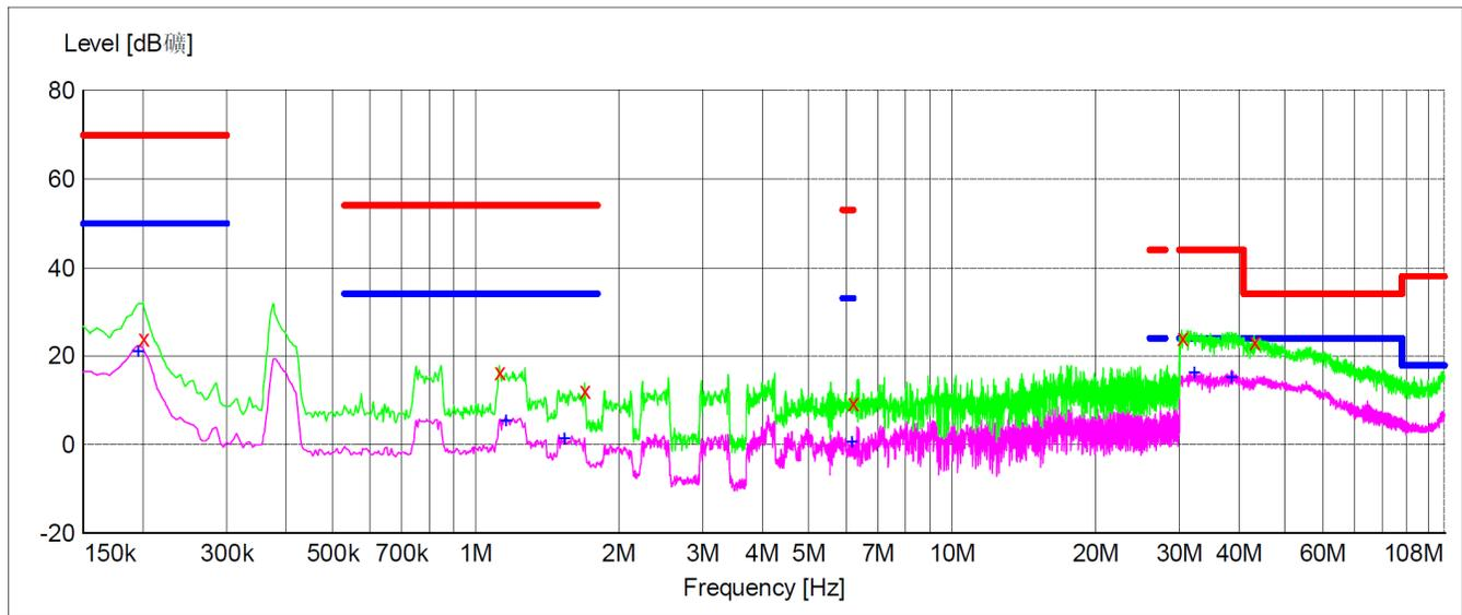
**Figure 17. EMC Conduction Test Result When the Device is Placed on Both Sides**
