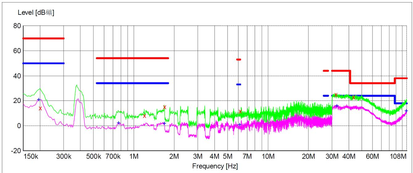
Figure 14. EMC Conduction Test Result When the Device is Placed on One Side
