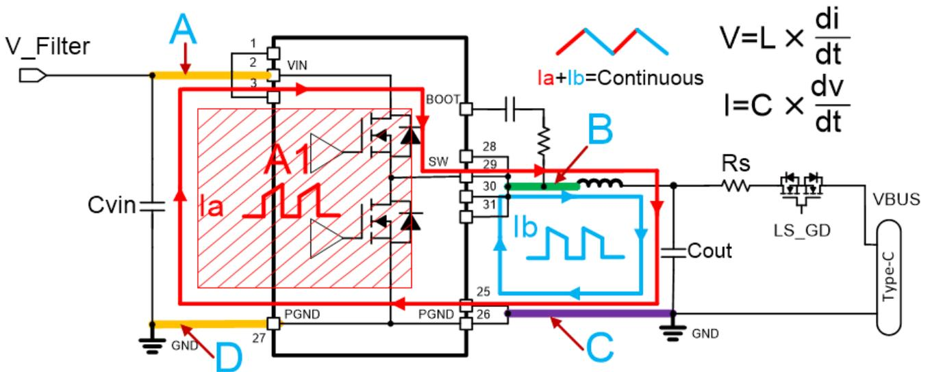
Figure 7. Buck Converter Schematic
