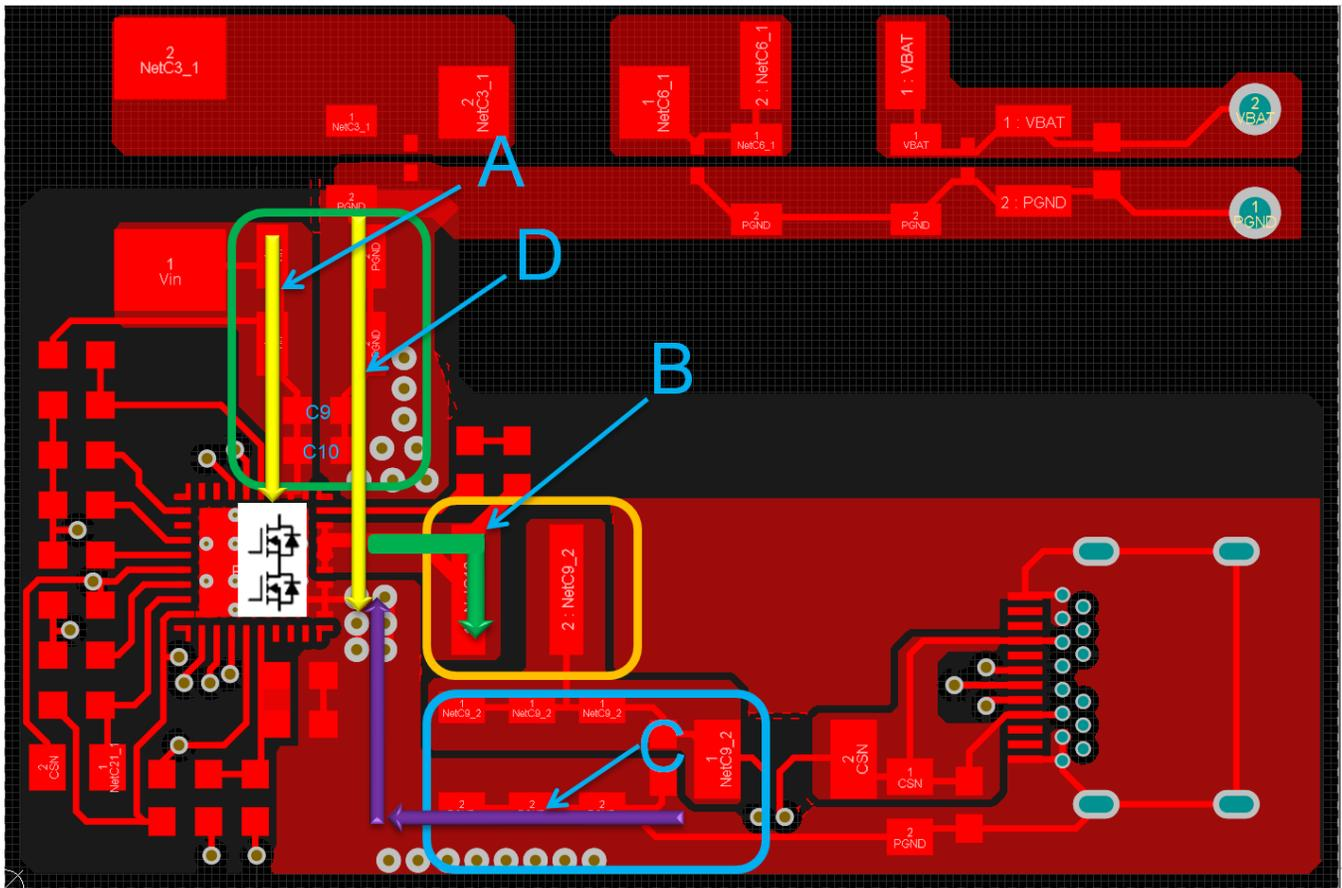
Figure 4. Common TPS2583X PCB Layout
