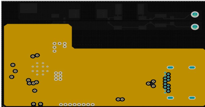
**Figure 10. Second Layer of the PCB Layout for the TPS2583X**
