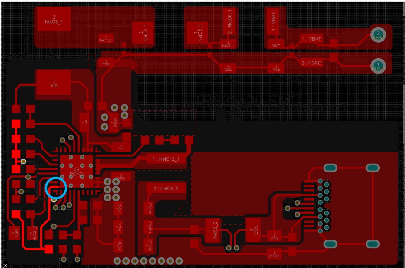
Figure 13. Bottom Layer of PCB Layout for TPS2583X
