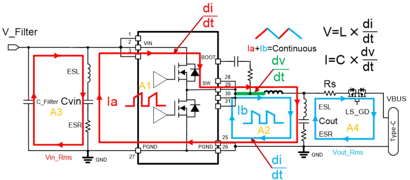
Figure 2. Topology of the Buck Converter and its Operating Principle
