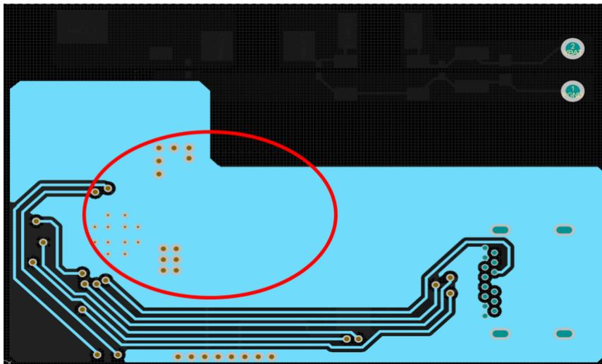
**Figure 11. Third Layer of the PCB Layout for the TPS2583X**
