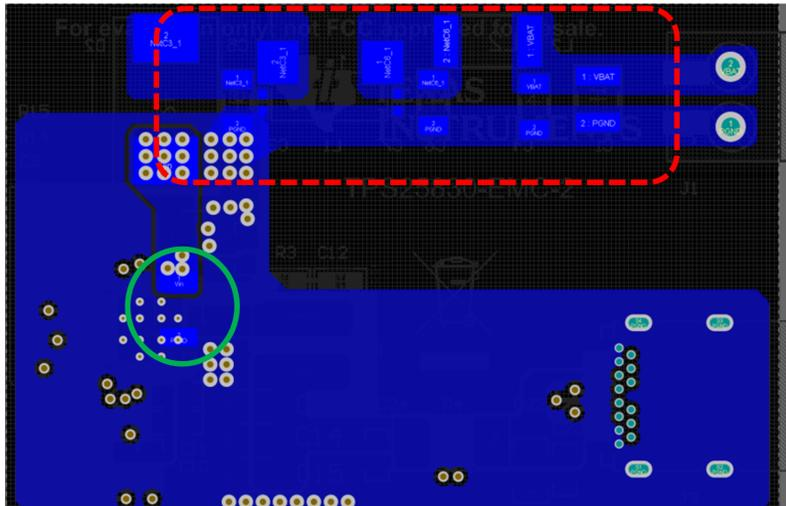
**Figure 15. Bottom Layer of the PCB Layout for Input Filter**
