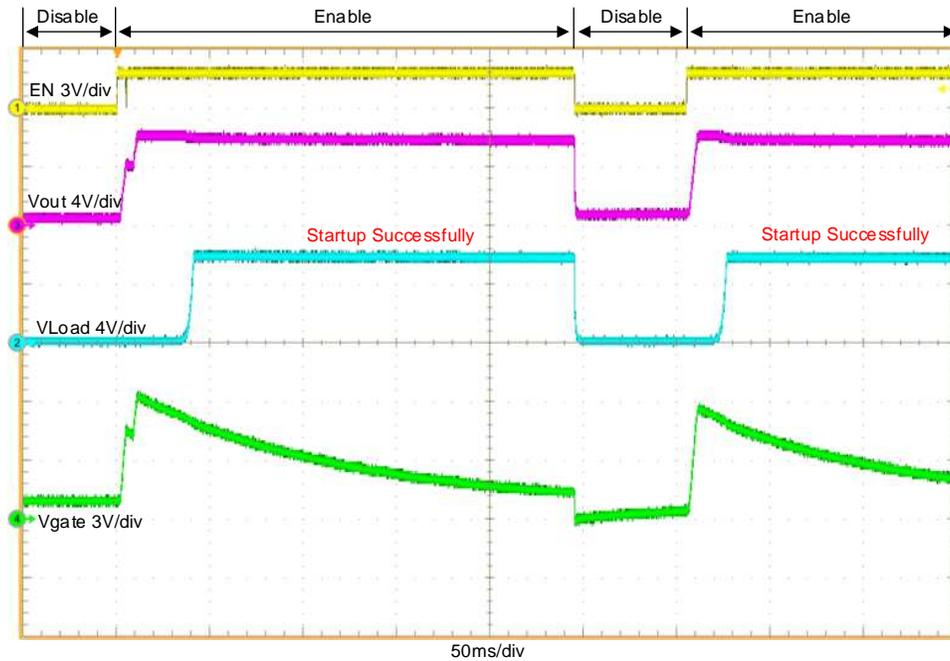
Figure 12. Quickly Restarts After Adding a Diode
