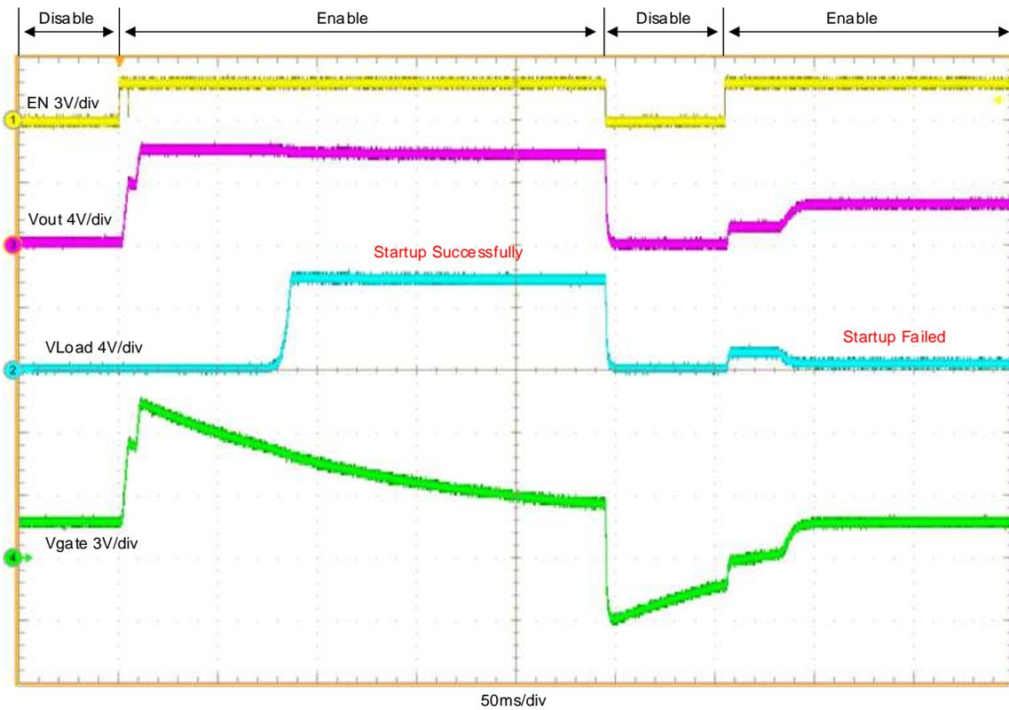
**Figure 10. Failed to Restart Quickly**
