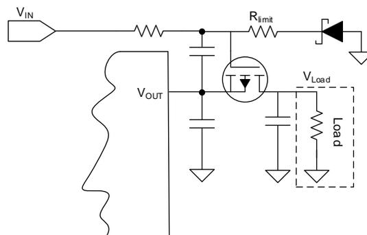
**Figure 11. The Circuit With a Diode to Discharge the  $C_g$**
