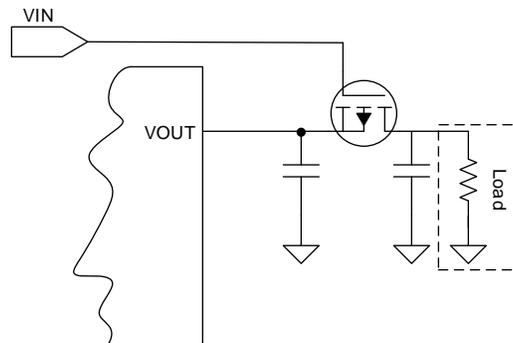
**Figure 7. The Circuit Using External FET Controlled by the Gap Between Vin and Vout**
