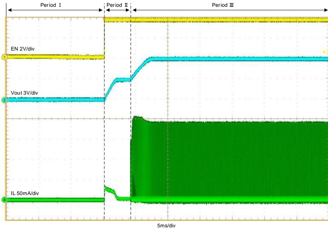
Figure 2. Start-up with 1 kΩ (Vin = 3.3 V)
