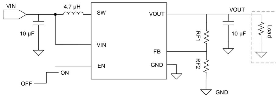
**Figure 1. Schematic of the TLV61046 Referred to EVM**
