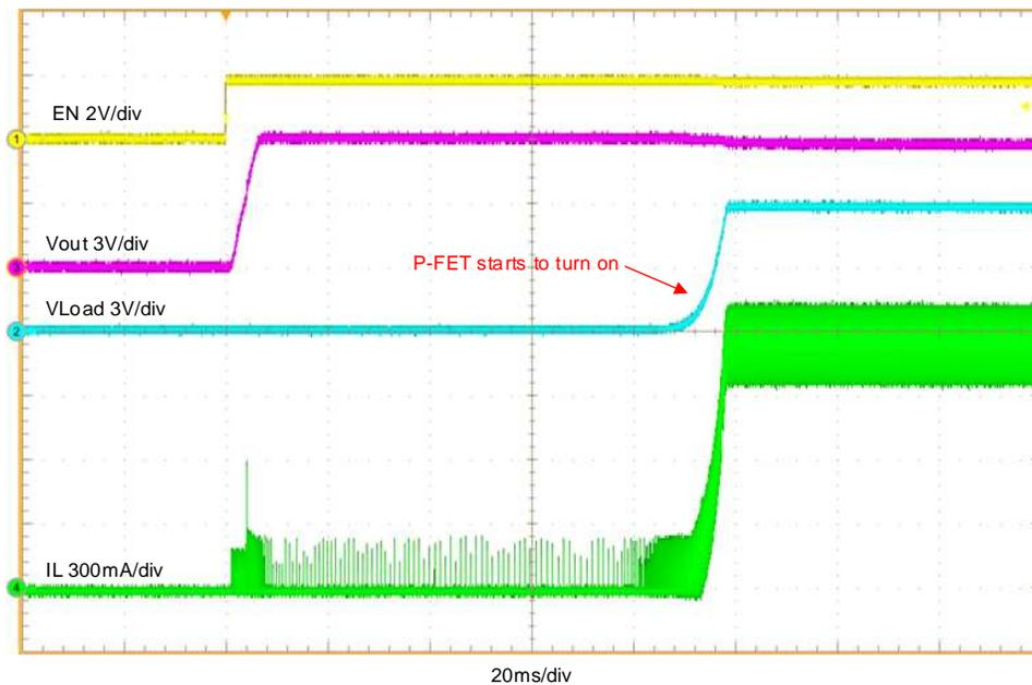
**Figure 9. The Solution 3 Circuit Start-up with 40  $\Omega$  and  $V_{in} = 1.8$  V**
