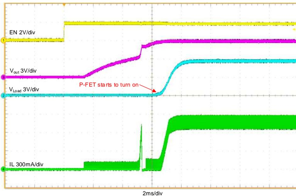
Figure 6. Circuit Start-up with  $40\ \Omega$  with  $V_{in} = 1.8$  V
