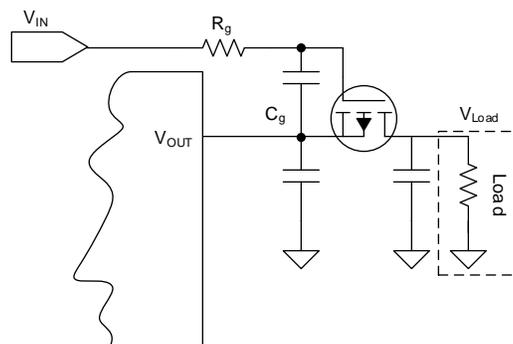
**Figure 8. The Circuit with an RC Delay Adding**
