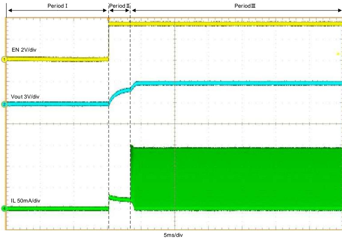
Figure 3. Start-up with 100 Ω Resistance Load (Vin = 3.3 V)
