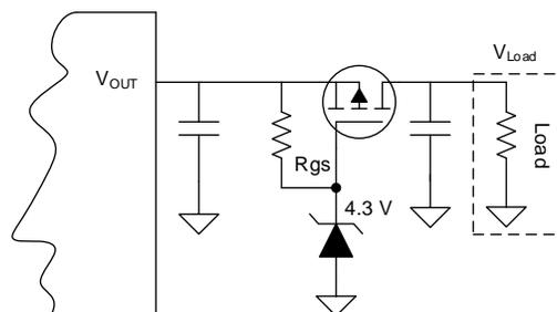
Figure 5. The Circuit with an External Fet and Zener Diode
