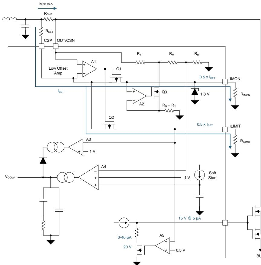
Figure 2. Cable Compensation Circuit
