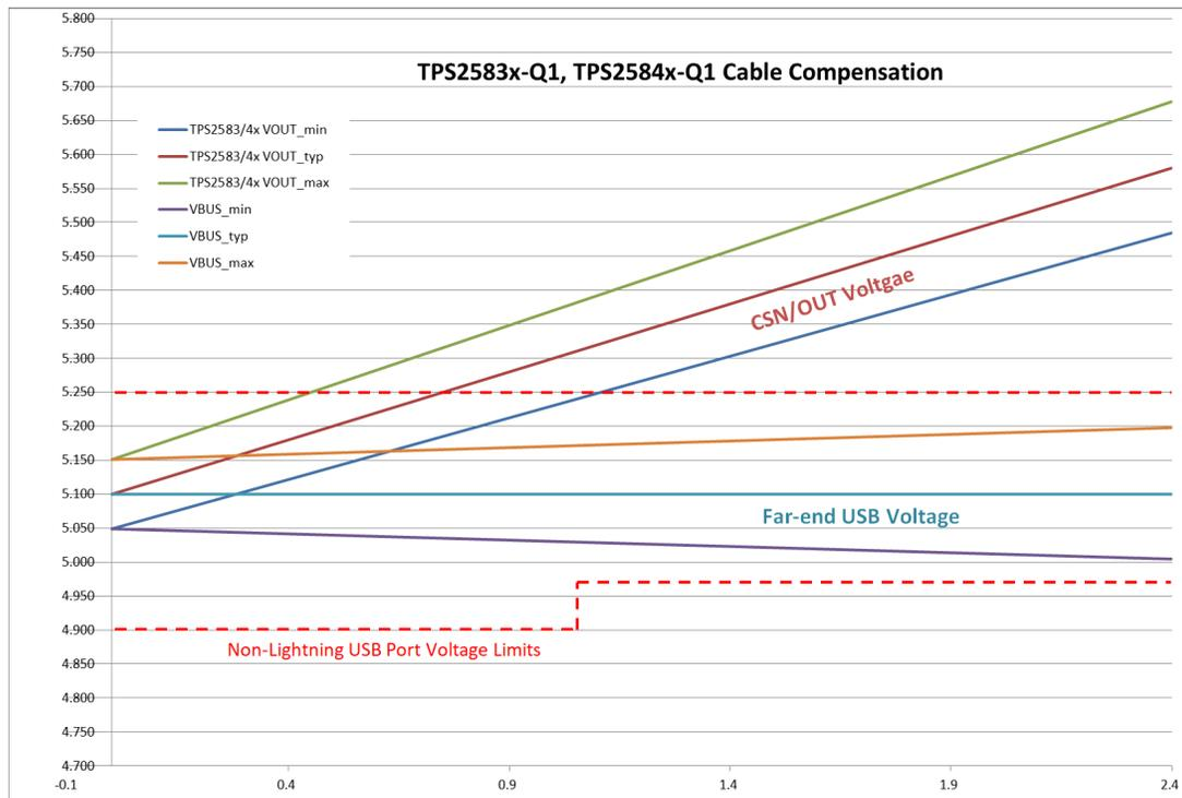
**Figure 3. TPS2583x-Q1 Far-end USB Voltage**
