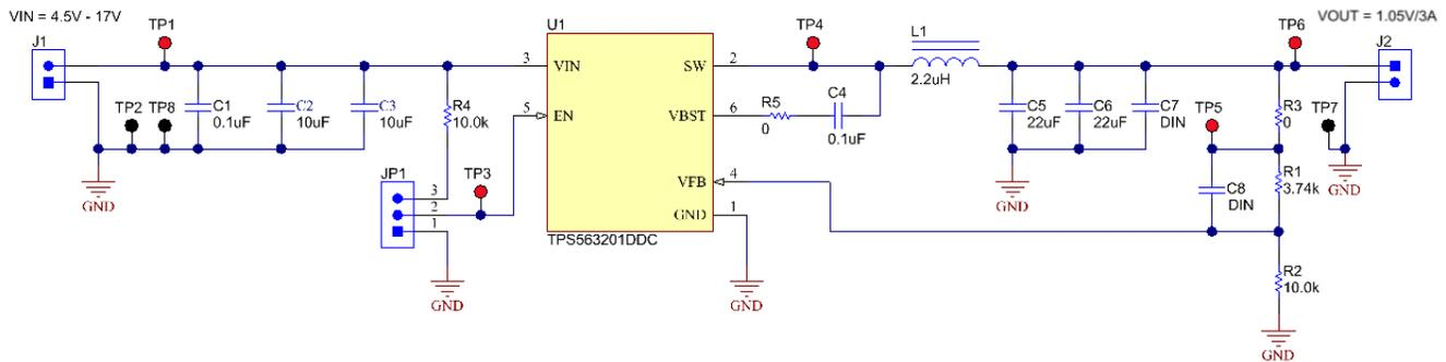
Figure 7. Schematic of the TPS563201EVM
