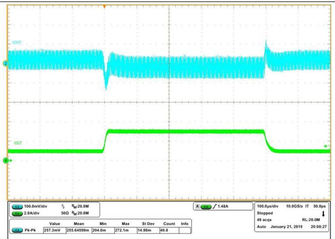
Figure 15.  $C_{out} = 10 \mu F$
