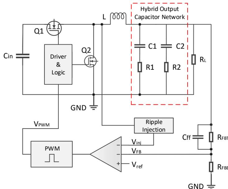
**Figure 26. The Hybrid Output Capacitor**
