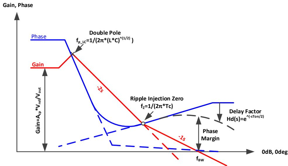
Figure 2. Bode Plot of the D-CAP2
