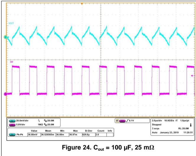
Figure 24.  $C_{out} = 100 \mu\text{F}, 25 \text{ m}\Omega$
