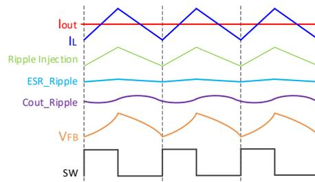
**Figure 4. Ripple Waveforms (Large Cout and Small ESR)**
