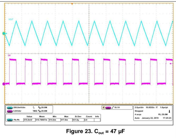
Figure 23.  $C_{out} = 47\ \mu\text{F}$
