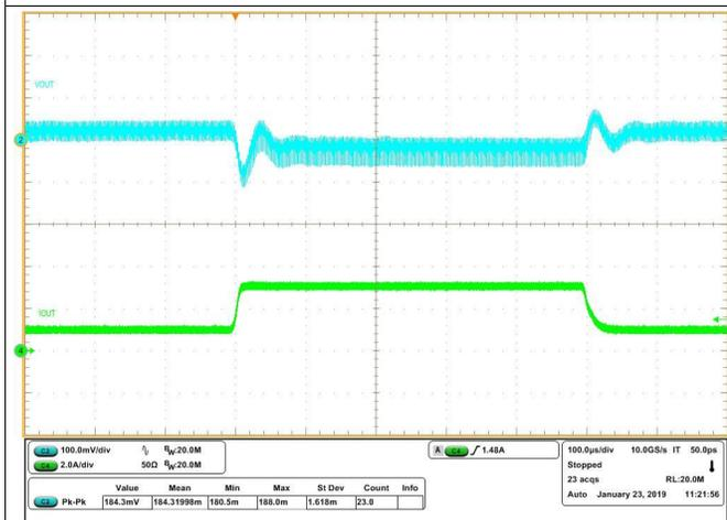
Figure 18.  $C_{out} = 100 \mu F, 25 m\Omega$
