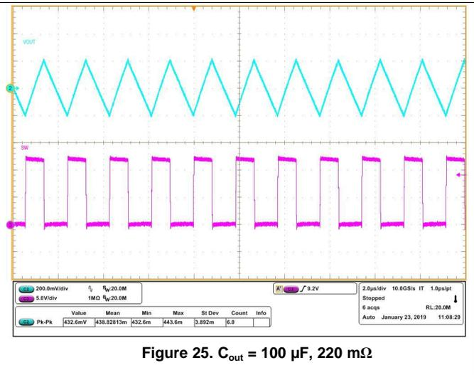
Figure 25.  $C_{out} = 100 \mu\text{F}, 220 \text{ m}\Omega$
