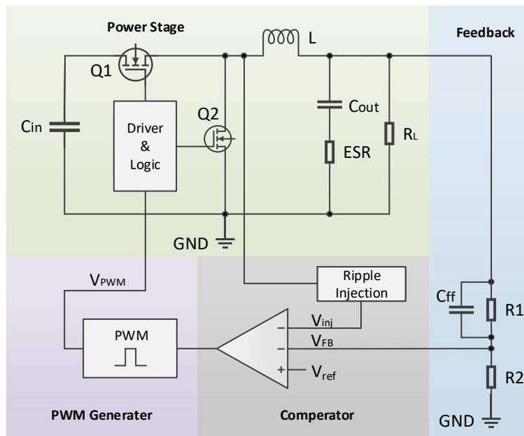
**Figure 1. The Block Diagram of the D-CAP2**
