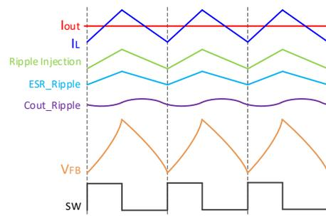
**Figure 5. Ripple Waveforms (Large Cout and Large ESR)**
