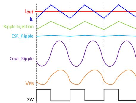
**Figure 6. Ripple Waveforms (Large Cout and Small ESR)**
