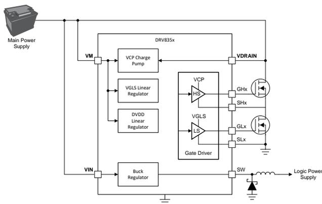
Figure 2. Single Supply Configuration
