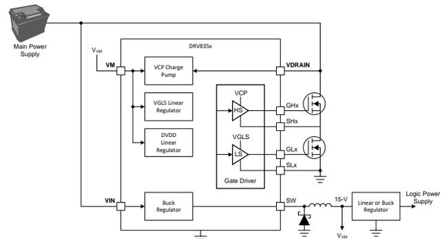
**Figure 3. Dual Supply Configuration**
