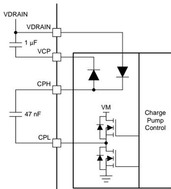
Figure 1. DRV835x Charge Pump Architecture
