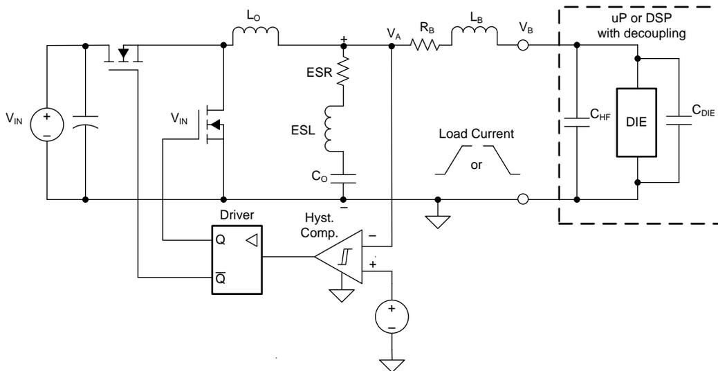
**Figure 3. Real-World Output Capacitor Arrangement[2]**
