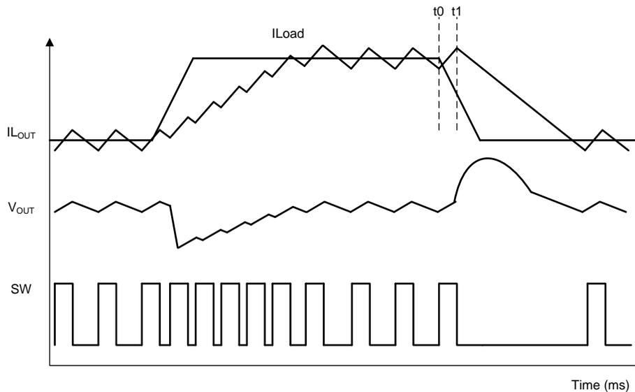
**Figure 2. Load Transient Response of D-CAPx Converter**
