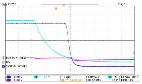
Figure 6. Scope Capture: System Entering Ship Mode
