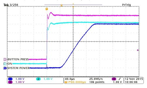
Figure 4. Scope Capture: System Exiting Ship Mode
