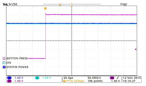
Figure 5. Scope Capture of Button Press: System Out of Ship Mode
