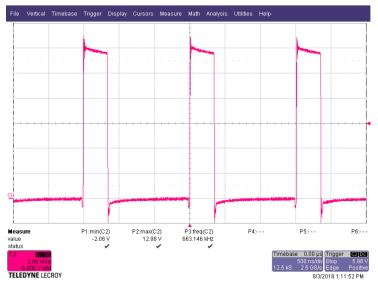
Figure 13. Switch Node Waveform – Layout 1
