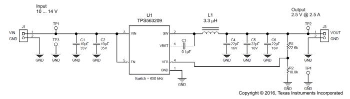
Figure 1. TPS563209DDCR 12 V to 2.5 V at 2.5 A
