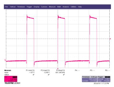
Figure 15. Switch Node Waveform – Layout 3
