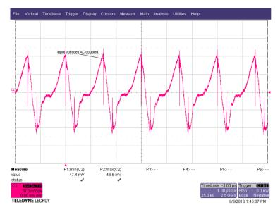
Figure 10. Input Ripple – 12 V to 2.5 V at 2.5 A, Layout 1
