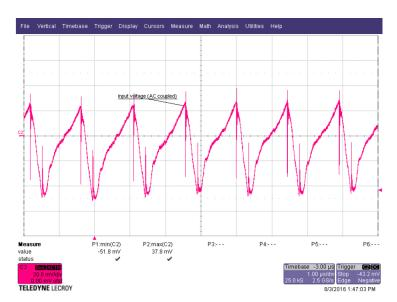
Figure 11. Input Ripple – 12 V to 2.5 V at 2.5 A, Layout 2
