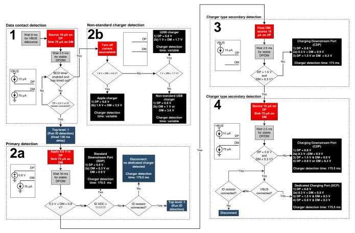
Figure 4. TSU6721 Charger Detection Flowchart
