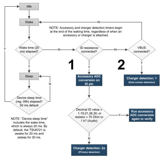
Figure 1. TSU6721 Top-level TSU6721 Detection Flowchart
