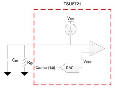
Figure 2. TSU6721 Simplified ADC Conversion Schematic
