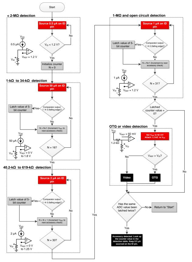
Figure 3. TSU6721 ADC Conversion Step for Accessory Detection on ID Pin
