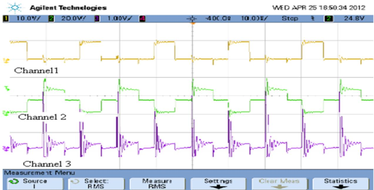
Figure 4. Gate Drive (Channel 1), Drain Voltage (Channel 2), Peak current (Channel 3), Respectively at 150 W
