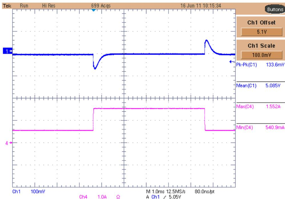
**Figure 11. Transient Response and Inductor Choice (0.5-1.5A step, 12μH)**
