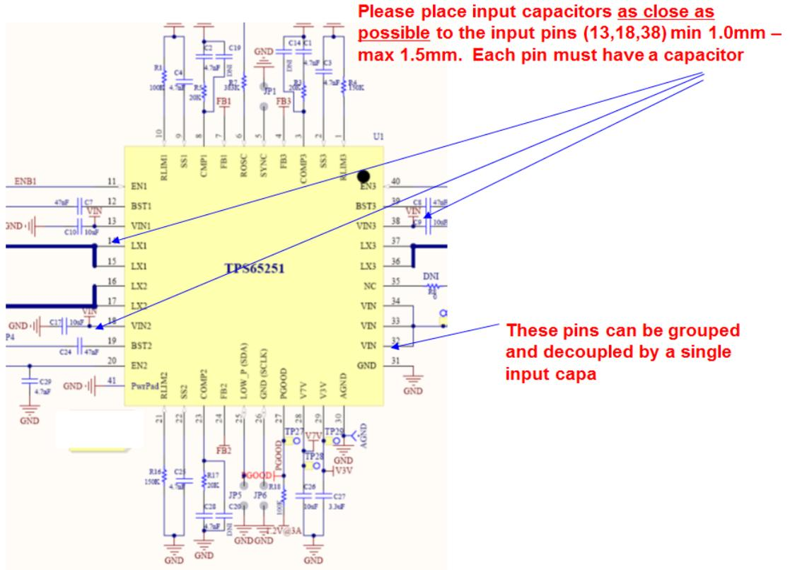
Figure 5. Capacitor Placement
