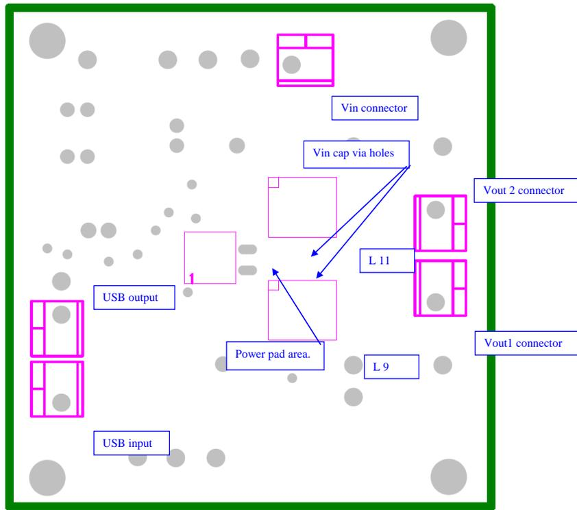
Figure A-11. TPS65252 Ground (2<sup>nd</sup>) Layer
