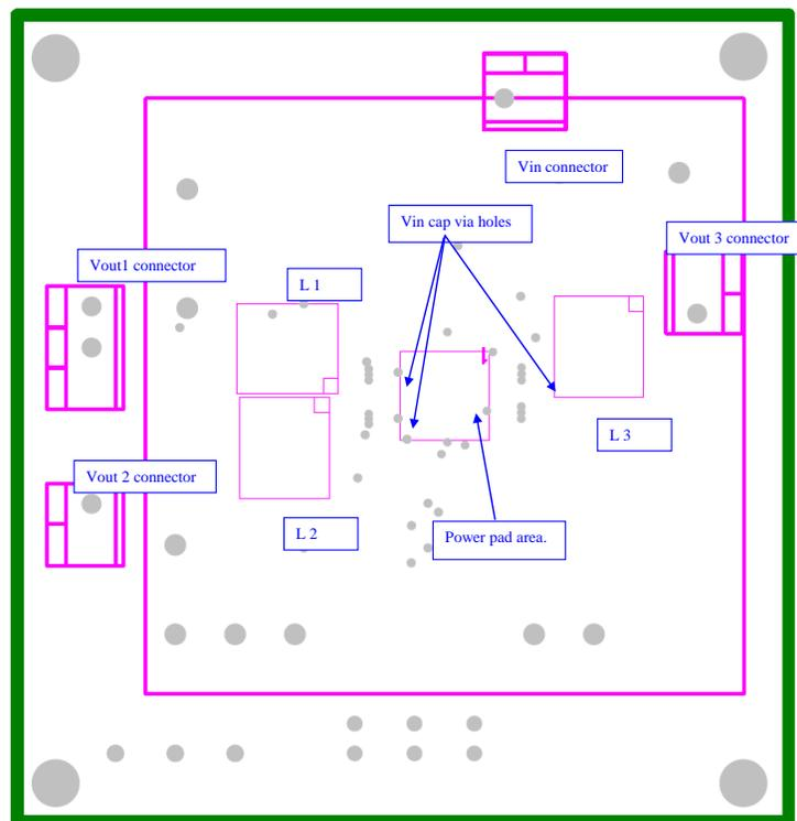
Figure A-2. TPS65251 Ground (2<sup>nd</sup>) Layer
