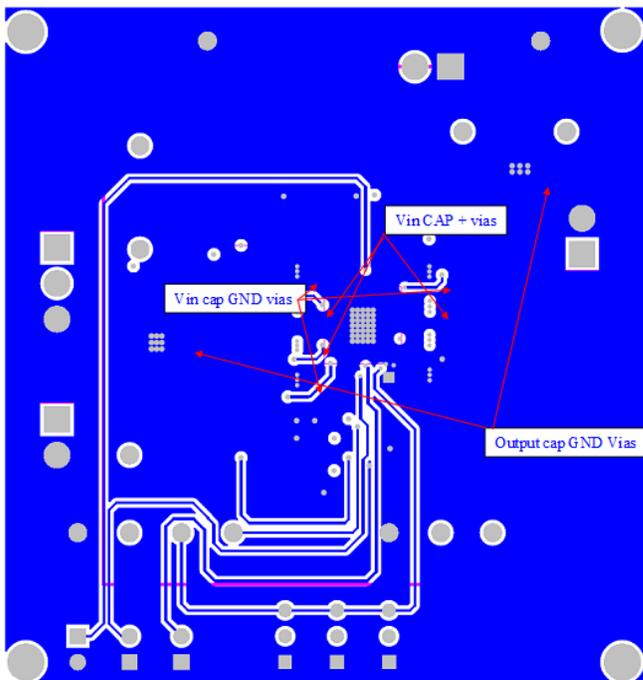
Bottom layer can be used to improve thermal dissipation by filling it with GND. Do not cut the GND plane area with traces near the TPS65251.
