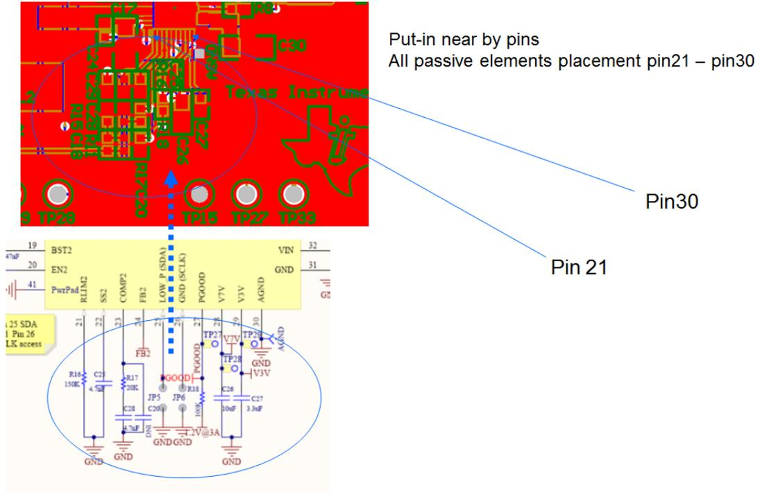
**Figure A-7. TPS65251 Placement Example 3**
