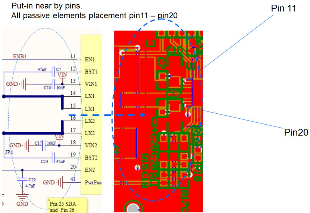
Figure A-6. TPS65251 Placement Example 2
