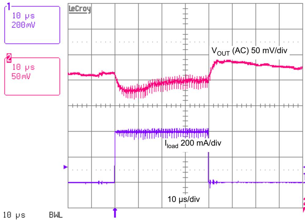
Figure 20. Load Transient Response 10 mA to 400 mA with  $V_{IN} = 12$  V
