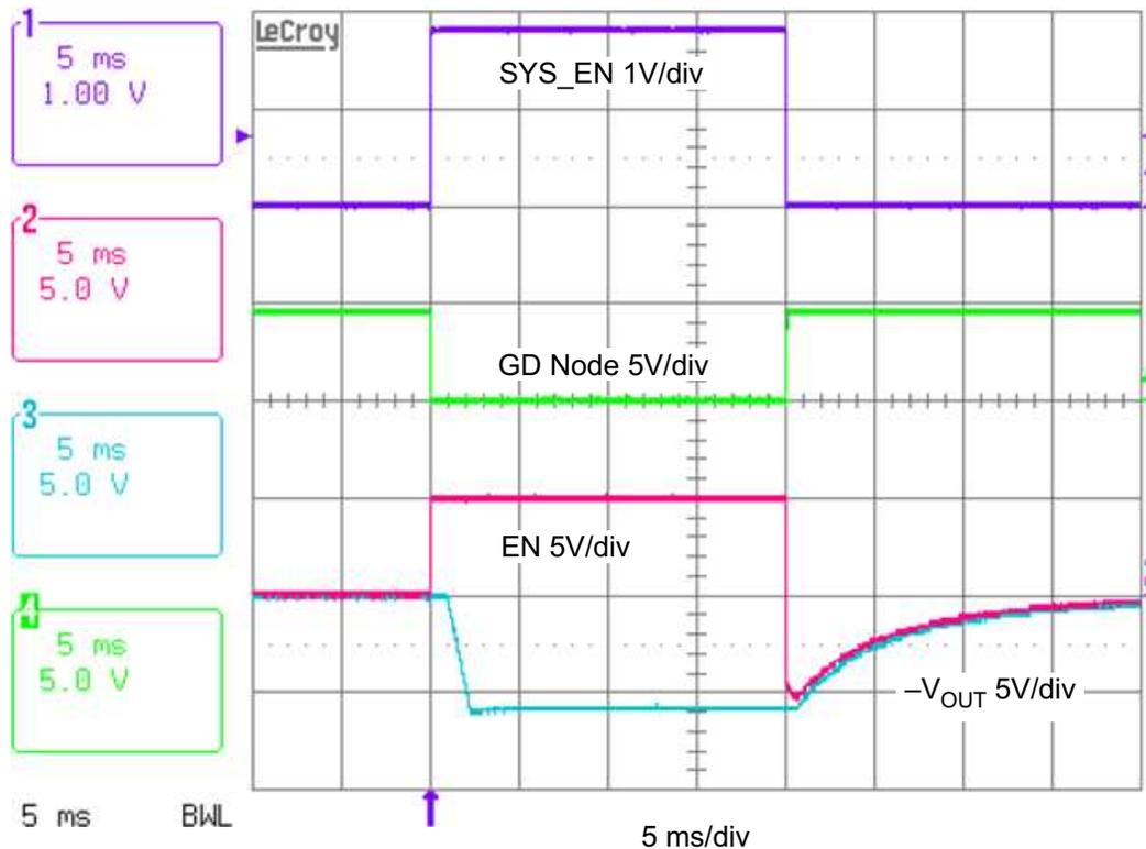
**Figure 6. EN Pin Level Shifter Test Results**
