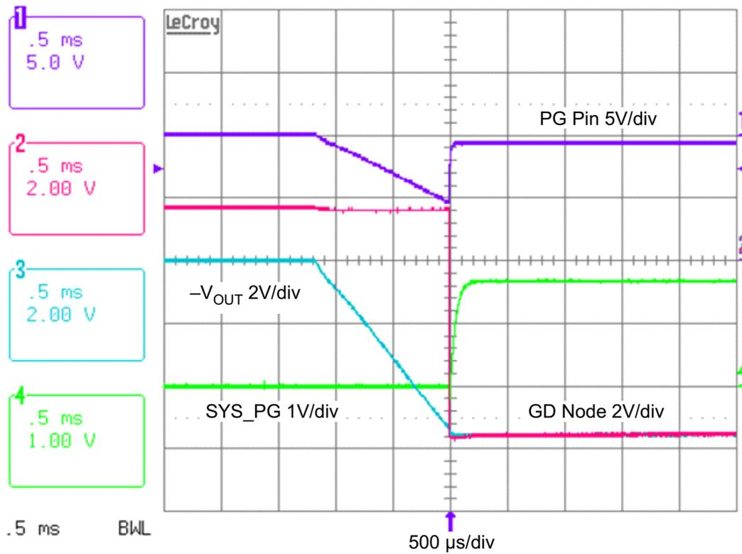
Figure 10. PG Pin Level Shifter on Startup
