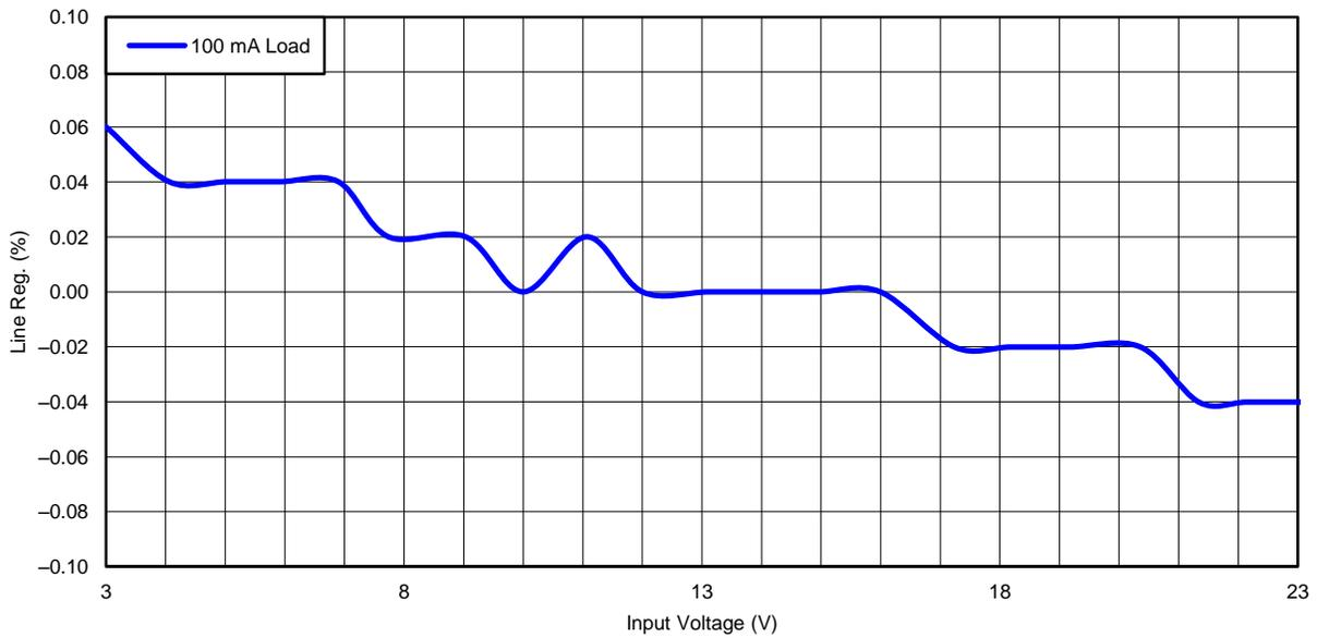
Figure 18. Line Regulation with  $V_{OUT} = -5\text{ V}$  and 100-mA Load
