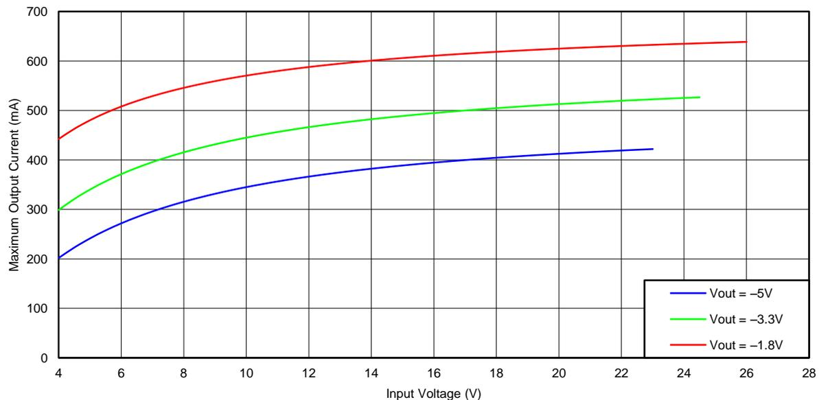
**Figure 4. Maximum Output Current vs.  $V_{IN}$**
