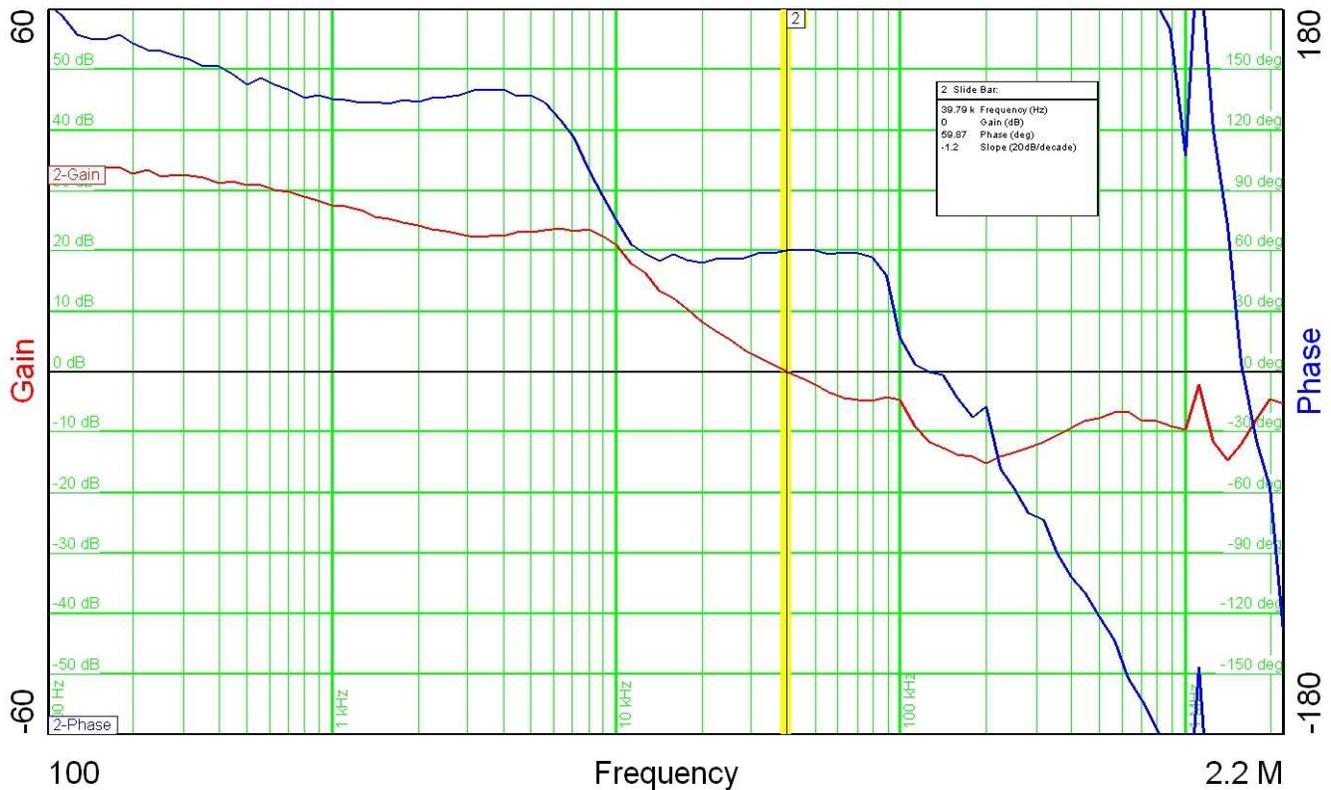
Figure 14. Bode Plot at 12-V  $V_{IN}$  and 400-mA Load
