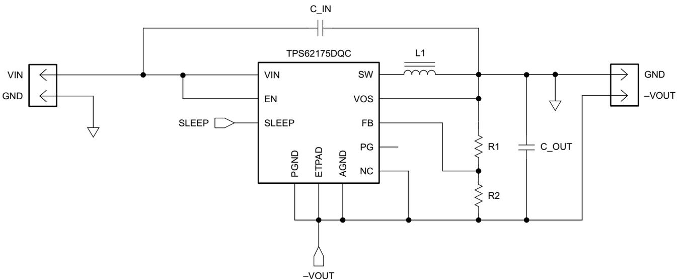
**Figure 2. TPS62175 Inverting Buck Boost Topology**
