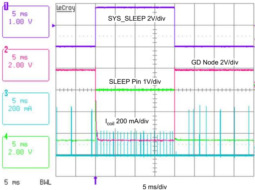
**Figure 8. SLEEP Pin Level Shifter Test Results**
