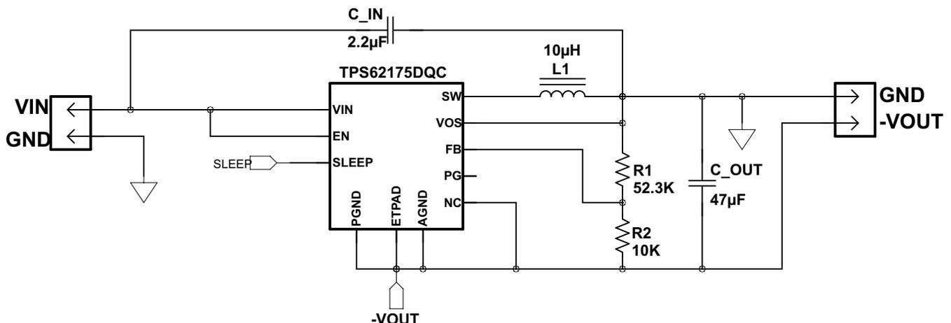
Figure 15. Schematic of Tested Circuit
