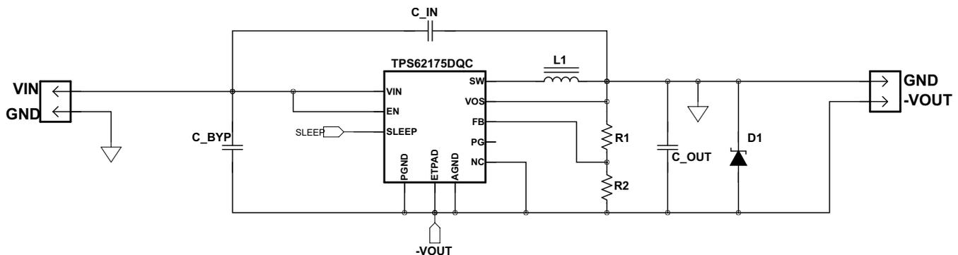
Figure 13. If Installing  $C_{BYP}$ , Installing Schottky D1 is Required
