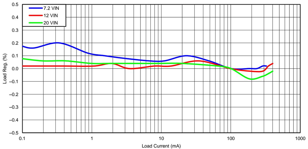
Figure 19. Load Regulation with  $V_{OUT} = -5\text{ V}$
