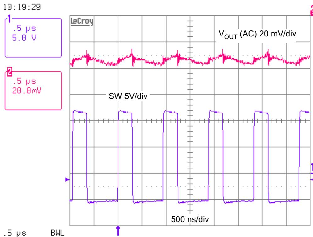
**Figure 22. Output Voltage Ripple,  $V_{IN} = 12$  V and  $I_{OUT} = 400$  mA**
