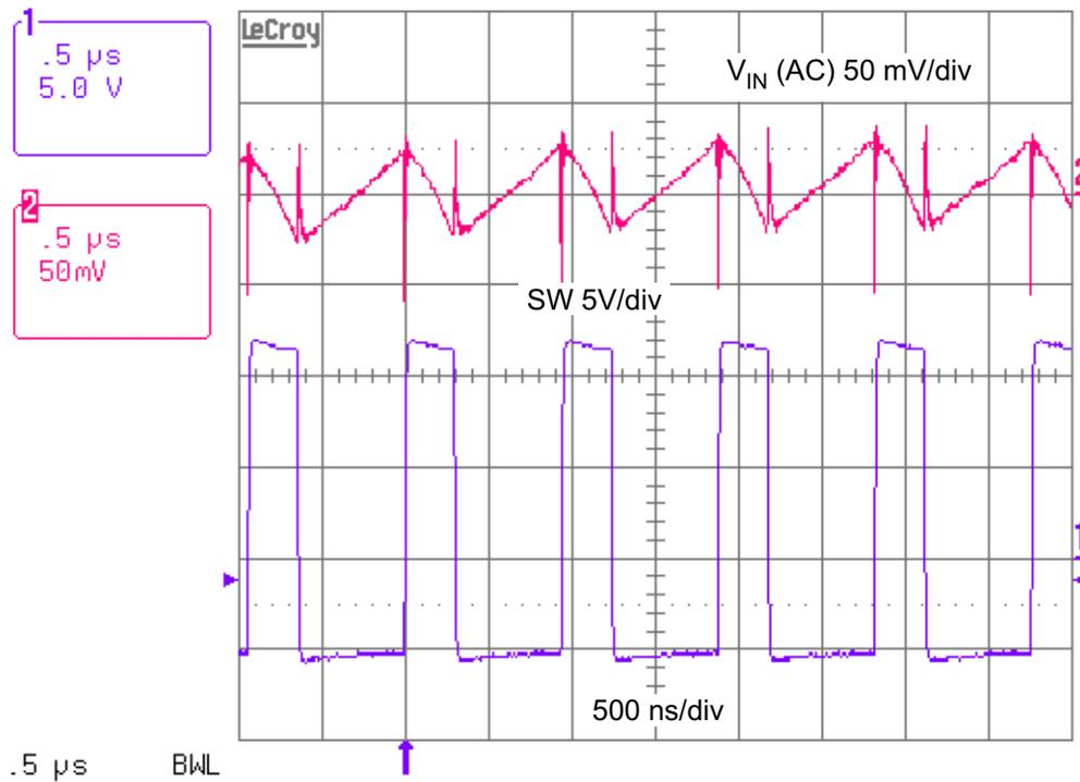
Figure 21. Input Voltage Ripple,  $V_{IN} = 12$  V and  $I_{OUT} = 400$  mA
