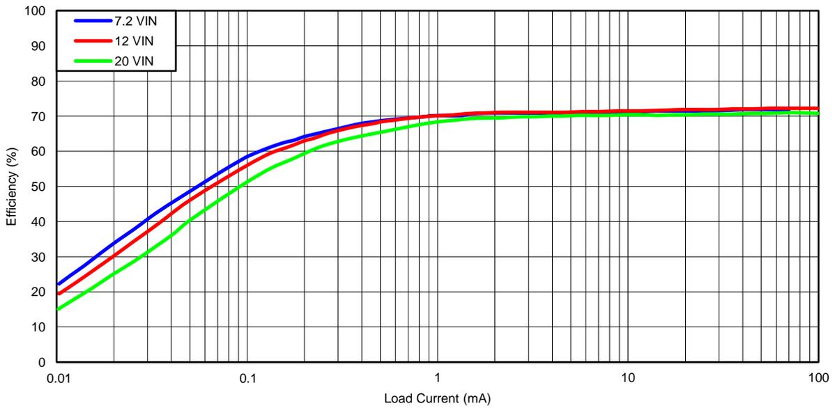
Figure 17. Sleep Mode Efficiency vs. Load Current with  $V_{OUT} = -5\text{ V}$
