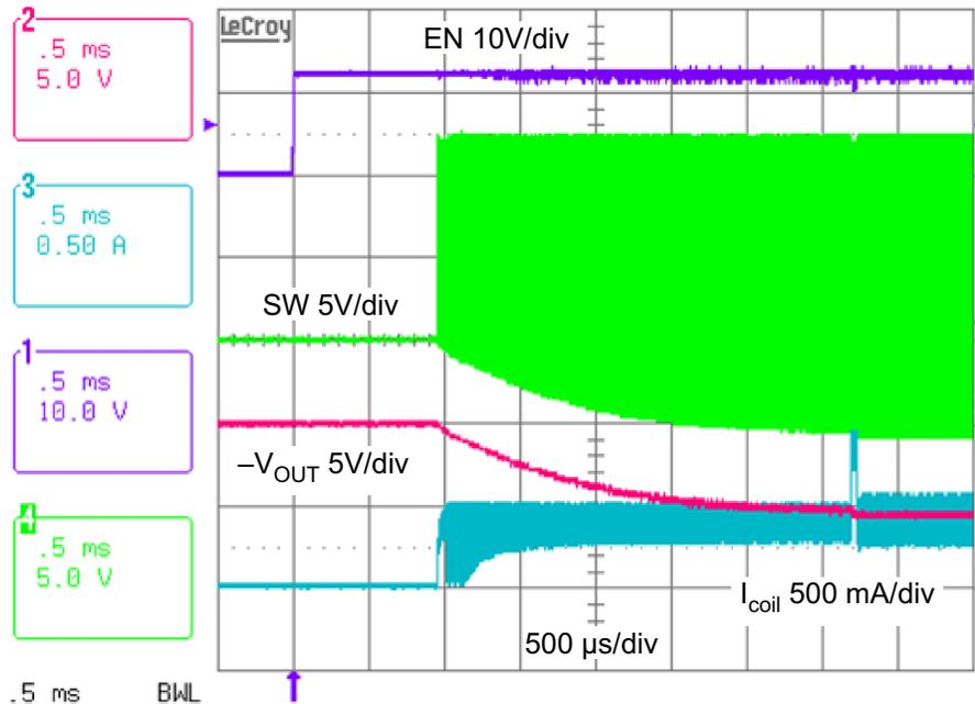
Figure 12. Startup on EN with 250-mA Load
