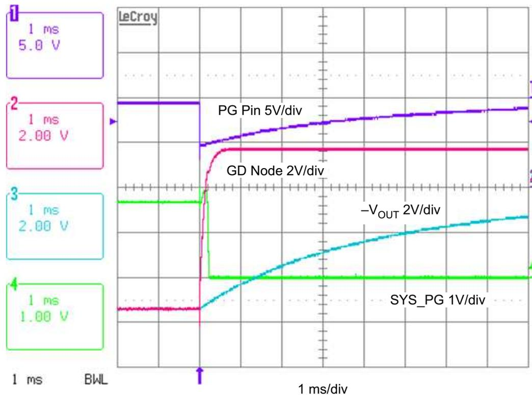
Figure 11. PG Pin Level Shifter on Shutdown
