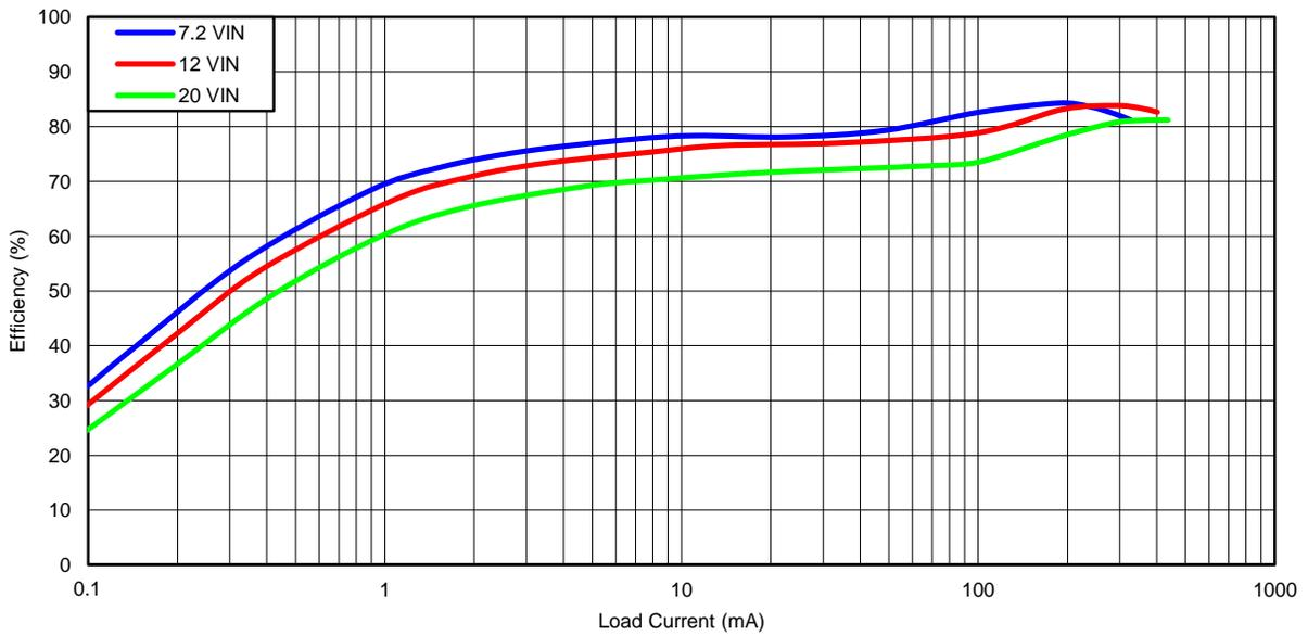
Figure 16. Normal Mode Efficiency vs. Load Current with  $V_{OUT} = -5\text{ V}$
