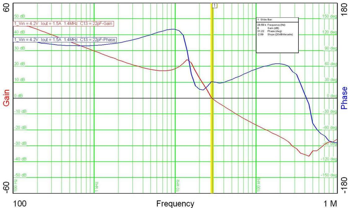
Figure 5. Control Loop Gain with 2.2- $\mu$ H Inductor and 100- $\mu$ F Capacitor
