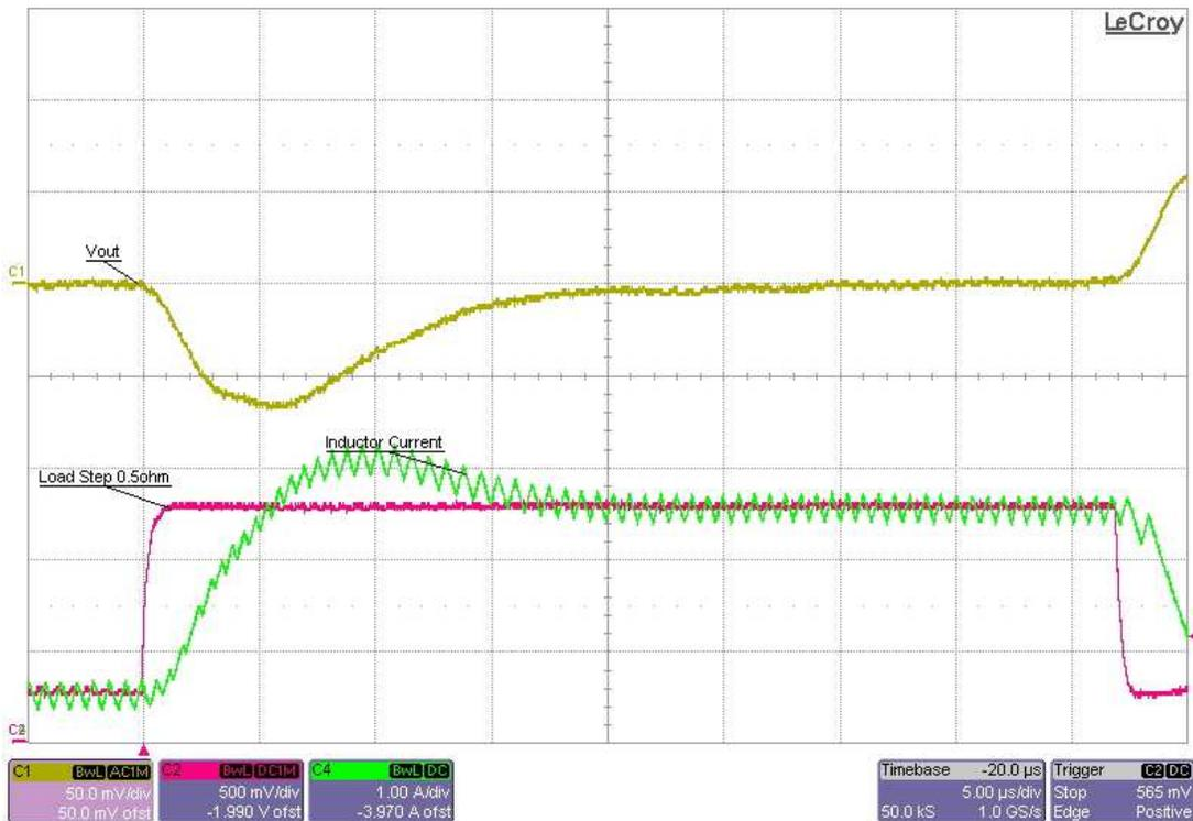
Figure 3. Load Transient with 2.2-µH Inductor and 100-µF Capacitor
