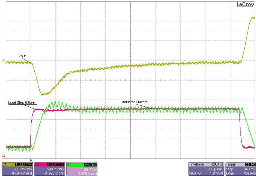
Figure 2. Load Transient with 2.2-µH Inductor and 10-µF Capacitor
