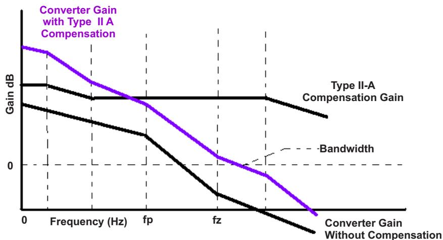
Figure 4. System Gain With Type II-A Compensation
