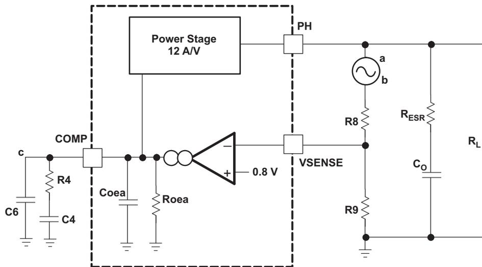
Figure 1. Small Signal Model for the Compensation Network
