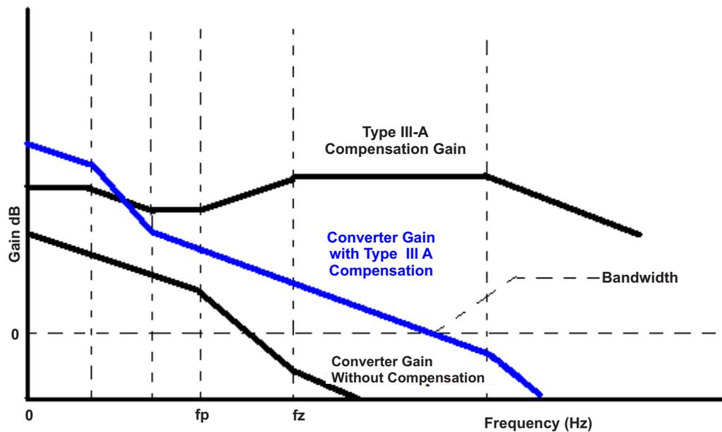
Figure 6. System Gain with Type III-A Compensation
