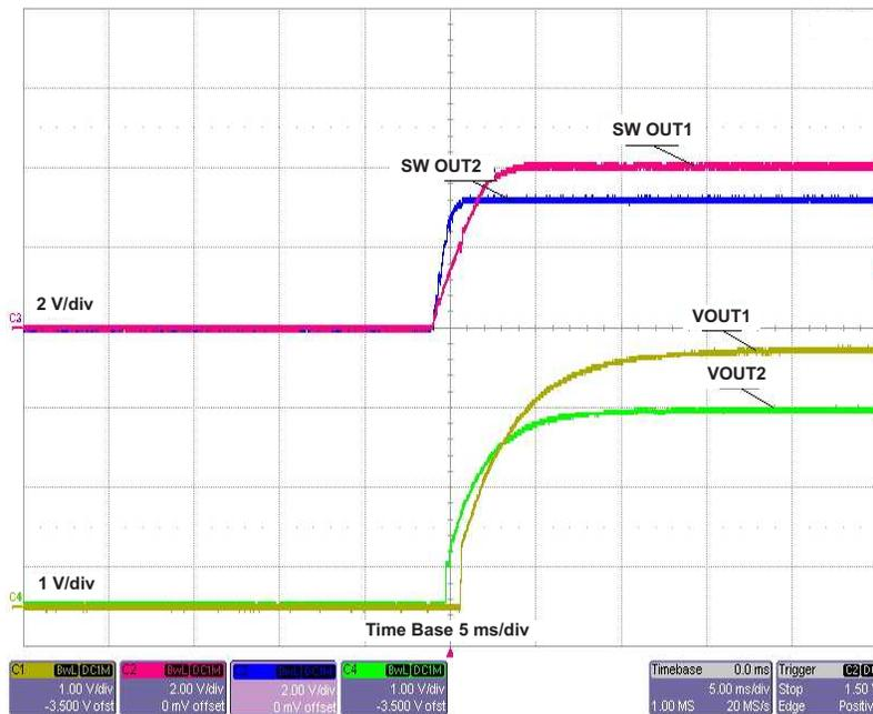
Figure 17. Ratiometric Start-Up With Vout2 Leading Vout1
