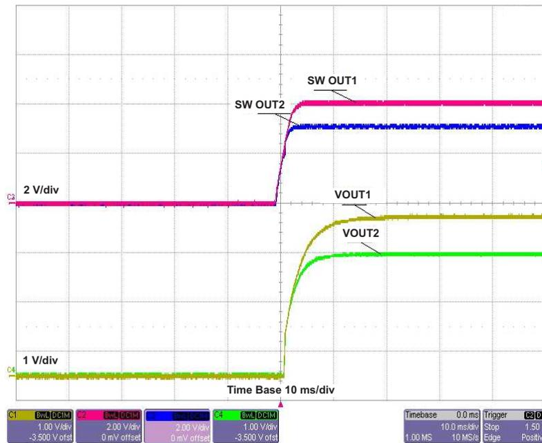
Figure 18. Simultaneous Start-Up
