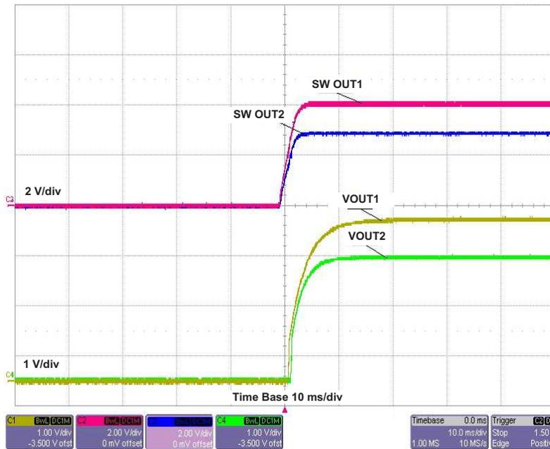
**Figure 16. Ratiometric Start-Up With Vout1 Leading Vout2**
