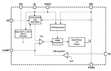
Figure 1. Internal Block Diagram of TPS61085
