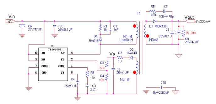
Figure 2. Schematic for 5V Isolated Power Supply with TPS61085
