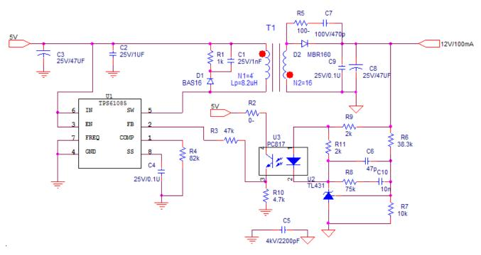
Figure 5. TPS61085 12V Isolated Solution with TL431 (Paper Design)
