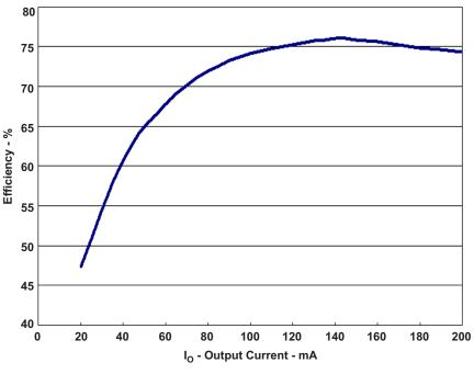
Figure 3. Efficiency with 5V Input
