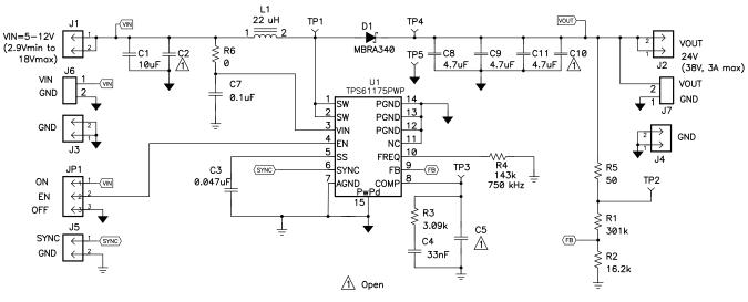
Figure 2. Schematic of TPS61175 EVM
