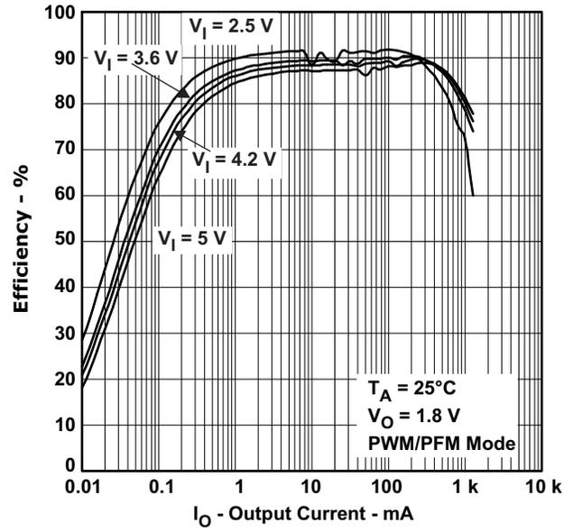
Figure 6. DCDC3: Efficiency vs Output Current
