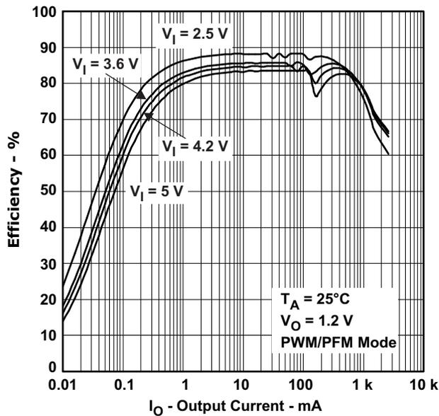
Figure 4. DCDC1: Efficiency vs Output Current
