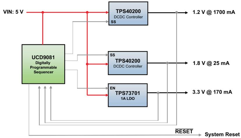
Figure 1. Block Diagram of Power Design
