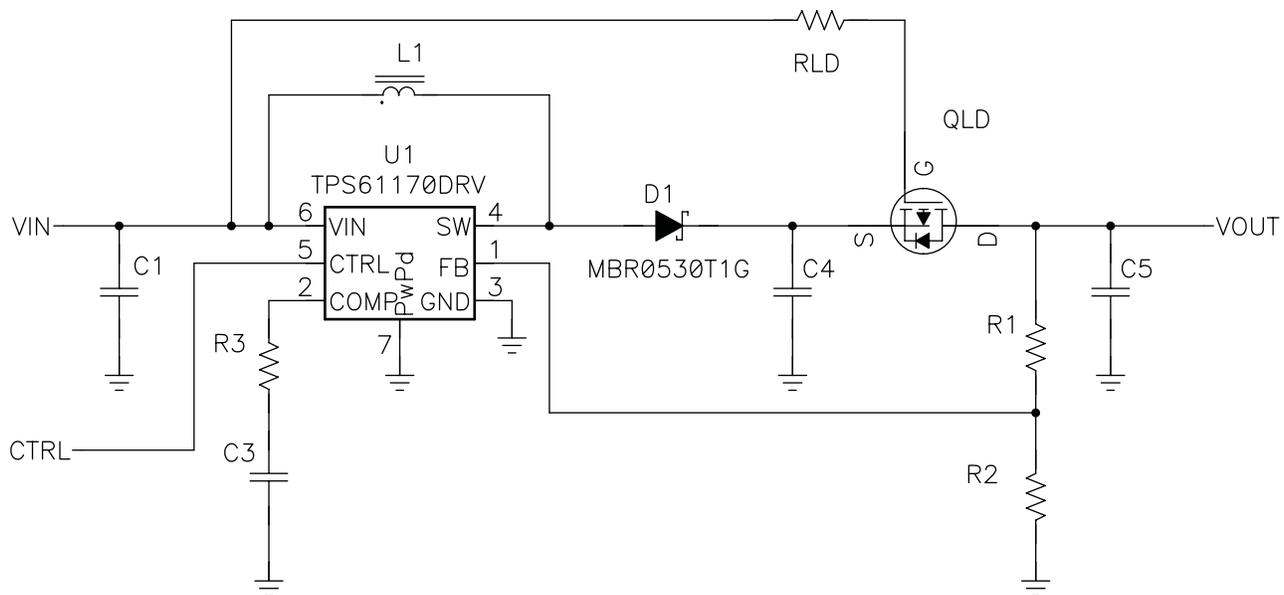
**Figure 1. TPS61170 with Input to Output Isolation**
