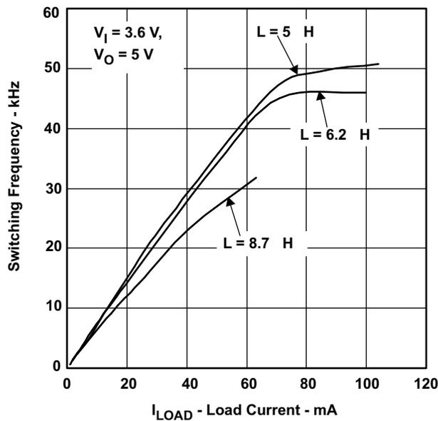
Figure 11. Inductor Effect on Switching Frequency
