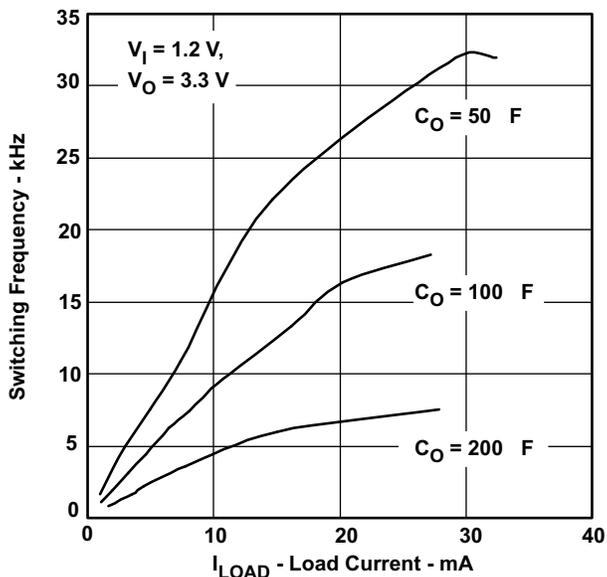
Figure 2. Output Capacitance Effect on Switching Frequency
