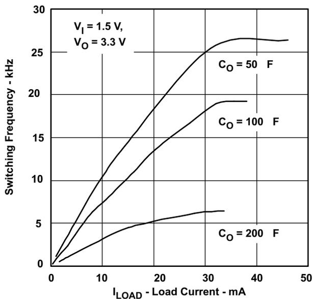
Figure 3. Output Capacitance Effect on Switching Frequency
