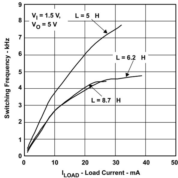
Figure 10. Inductor Effect on Switching Frequency
