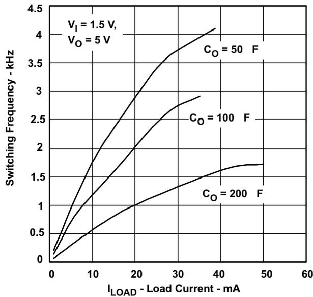
Figure 5. Output Capacitance Effect on Switching Frequency
