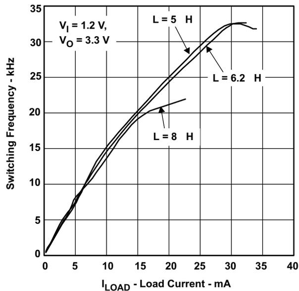
Figure 7. Inductor Effect on Switching Frequency
