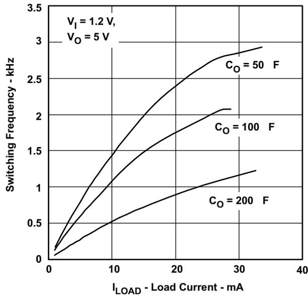
Figure 4. Output Capacitance Effect on Switching Frequency
