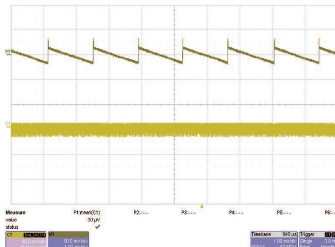
**Figure 1. PSM Output Ripple (Top Waveform) 50 mV/div vs PWM Output Ripple (Bottom Waveform) 50 mV/div**
