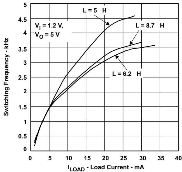
Figure 9. Inductor Effect on Switching Frequency
