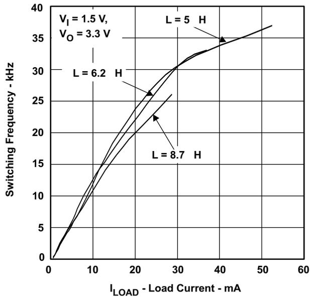
Figure 8. Inductor Effect on Switching Frequency
