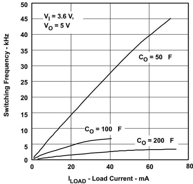
Figure 6. Output Capacitance Effect on Switching Frequency
